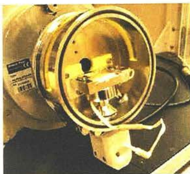
Figure 3.8: Anton Parr TTK450 heating and cooling stage used for variable temperature XRPD.
