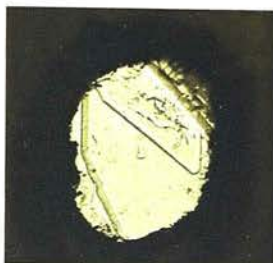
Figure 4.7: Optical image of two single crystals of DMU (form IV) in a diamond-anvil cell at 0.9 GPa
