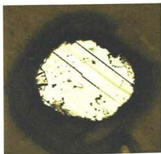
Figure 4.6: Optical image of single crystal of DMU (form III) in a diamond-anvil cell at 0.7 GPa.
