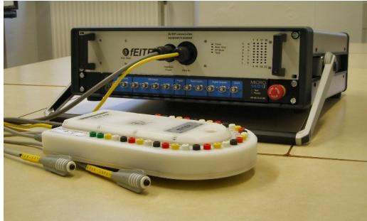
Figure 2-6 fEITER system: base unit and head box (the white box)
