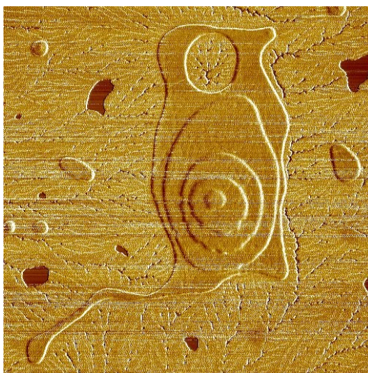
AFM phase image of a symmetric poly(isoprene- b -ethylene oxide) PI- b -PEO thin film spin cast on mica (the size of the image is 20 \times 20 \mu\text{m}^2 ).
