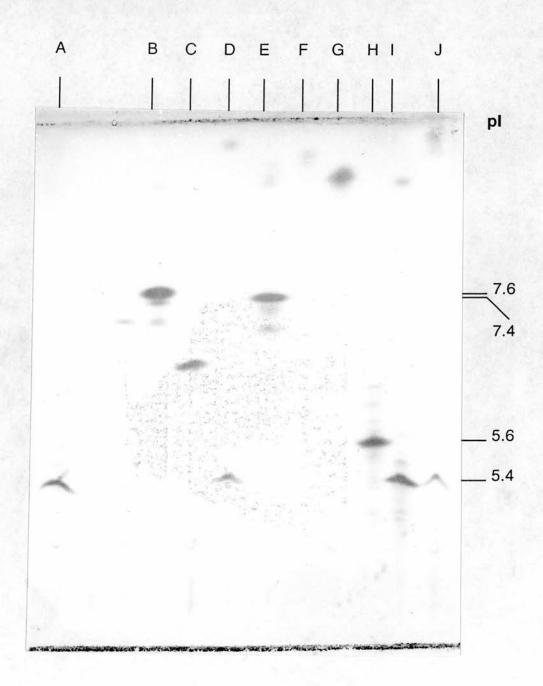
Figure 12. Analytical iso-electric focusing of  $\beta$ -lactamases isolated from wild type, non-transferable ampicillin resistant strains in Edinburgh
