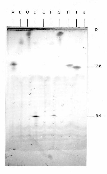
Figure 13. Analytical iso-electric focusing of  $\beta$ -lactamases isolated from wild type, non-transferable ampicillin resistant strains in Edinburgh
