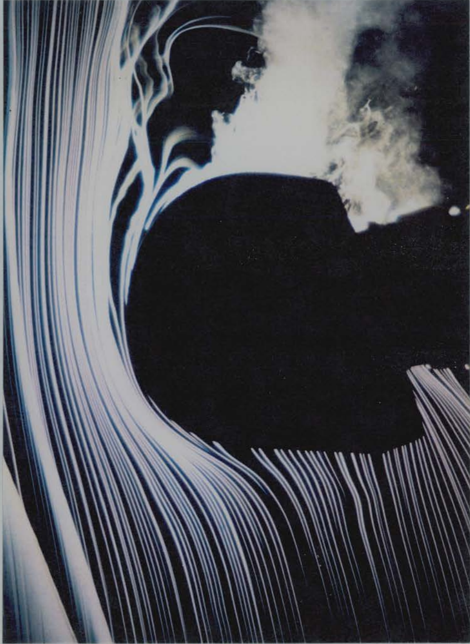
FIGURE 2.9 AIRFLOW PATTERN AROUND MOTORCYCLE HELMET (SMOKE IN WIND TUNNEL) COURTESY OF D. NASH.
