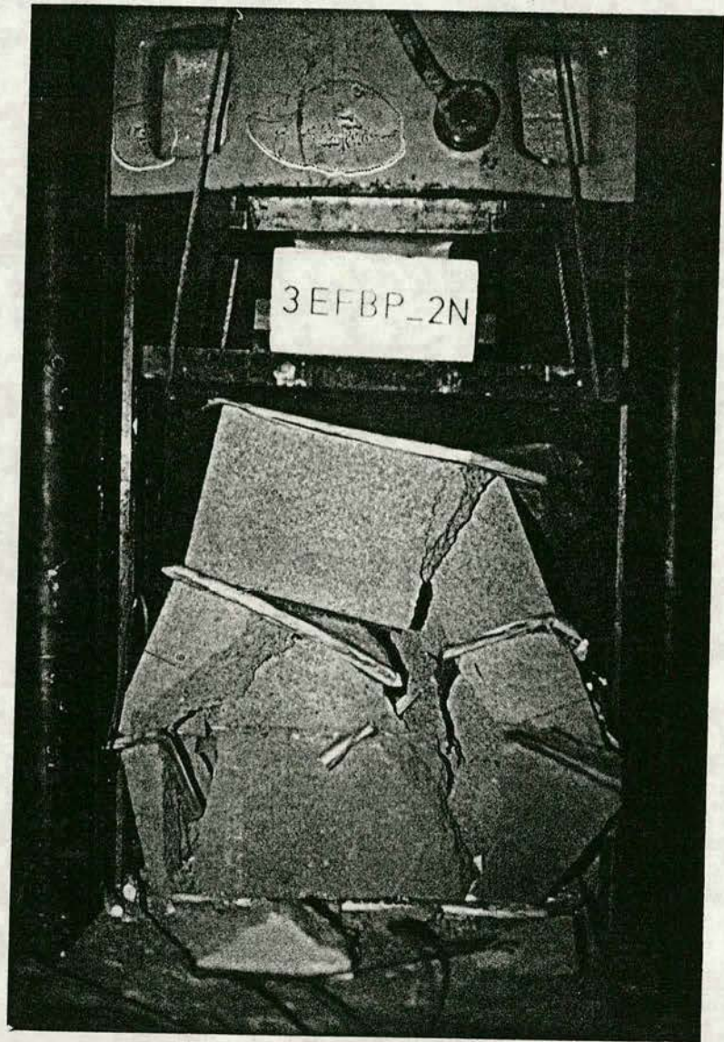
Fig. 5.5 - Unfilled 3FBP-DPJ prism after failure.
