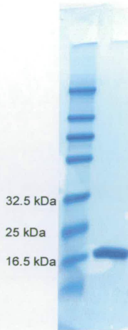
Figure 3:13 SDS PAGE of purified deglycosylated MCP12. The gel shows that MCP12 has been purified to homogeneity, as judged by SDS PAGE and runs at approximately the correct molecular weight for MCP12.
