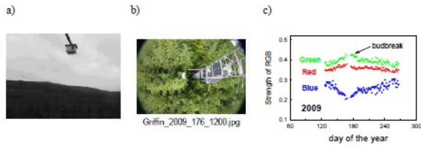
Fig. 2 The camera installed in Griffin, Perthshire (a), the canopy image of Sitka spruce (b) and the strength of colour signals (c). Unfortunately, the observation has stopped due to power failure since October 2009.
