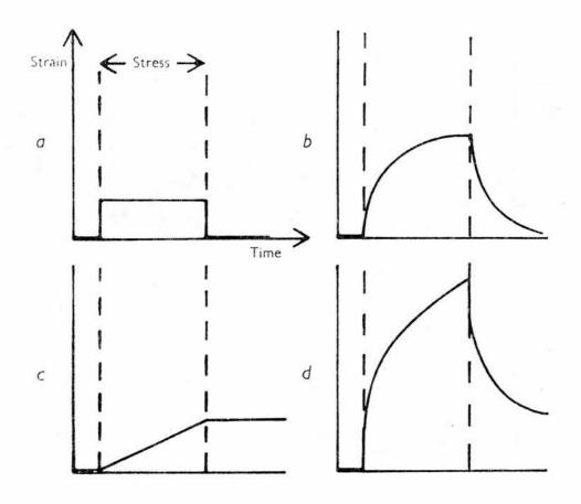
Fig. 2.6 Strain (displacement) of a visco-elastic material in response to a stress (force) applied between the dotted lines: (a) instantaneous elastic strain, (b) slow elastic strain, (c) viscous flow (creep). At (d) the overall response of the material is shown. From Alexander (1968).
