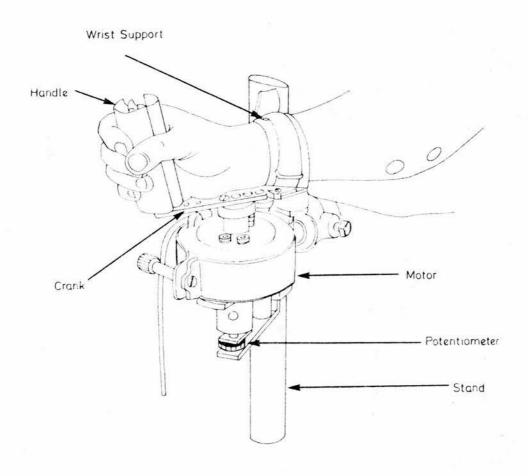
$\overline{\text{Fig. 2.4}}$  The G9M4 motor is shown in use at the wrist. The arrangement for coupling the limb to the motor is shown, and the site of attachment of the forearm flexor EMG electrodes is indicated.
