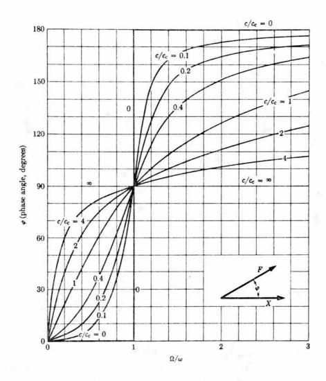
Fig. 2.8 The phase angle between force and displacement. This figure illustrates that, regardless of damping, the phase angle is 90°, when the ratio of driving force frequency to the natural frequency of the system is 1, i.e. at resonance. As the velocity vector leads the displacement vector by 90°, the phase angle between torque and velocity at resonance is 0°. From Burton (1968).
