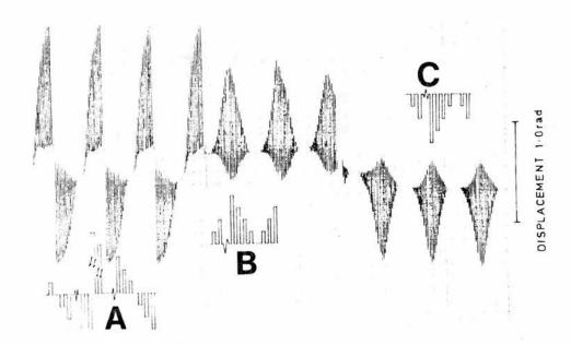
Fig. 3.33 Ramped monophasic torque pulses. In this series of experiments the applied torque did not alternate into flexion and extension, but the torque acted in only one direction, becoming zero between pulses. The displacement only was recorded, but the pattern of applied torque is shown (not to scale).
