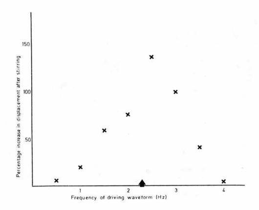
Fig. 3.24 Influence of frequency on "thixotropic" response. The percentage increase in amplitude following the application of 4 or 5 cycles of square wave stirring torque at 0.4 N m. The driving torque was held constant at 0.08 N m. These results would have been different if the driving force had been adjusted to maximise the effect at each frequency. The resonant frequency is indicated by an arrow.
