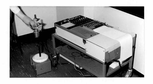
Fig. 2.1 The waveform generator/power amplifier/chart recorder unit and the G6M4 motor are seen in use at the wrist.
