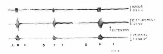
Fig. 3.23 "Driving force" and "stirring force". At "A" a small sinusoidal force (driving force) at 3.0 Hz is applied to the wrist. "Stirring" with a sinusoidal force of 4 times the size "B" causes a transient increase in amplitude "C". Increasing the size of the driving force slightly "D" gives a sustained increase in amplitude "F", even though the stirring force "E" is only applied for 2 cycles.
