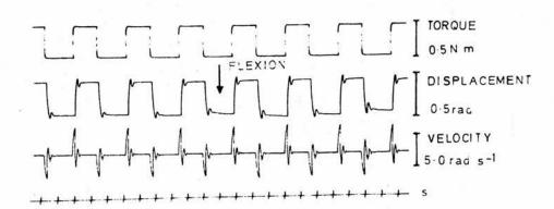
Fig. 3.27 Rectangular torque pulses. An alternating rectangular torque is applied to the wrist. The wrist follows the applied torque; overshoots and decrementing oscillations are seen in the displacement record. The wrist is evidently less than critically damped. The velocity with which the wrist moves is determined by its viscous resistance.
