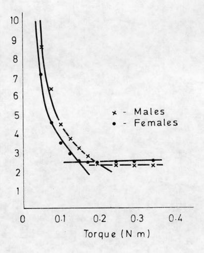
Fig. 3.10 "Mean curves" for male and female subjects. The mean values of resonant frequency of the wrist are plotted at 10 torque levels. The standard error for differences in the mean is 0.292. Thus the curves become significantly different (p < 0.05) at 0.15 N m and lower torques, and are not significantly different with larger torques. The mean torque thresholds for men and women are 0.22 N m and 0.14 N m respectively.
