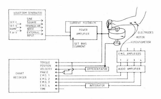
Fig. 2.2 A block diagram of the experimental apparatus.
