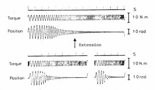
Fig. 3.6 Effect of sweep rate on resonance. The frequency was logarithmically swept from 0.5 Hz to 16 Hz at a rate of  $\frac{1}{3}$  8 vs  $^{-1}$ ,  $\frac{2}{3}$  8 vs  $^{-1}$ , and  $\frac{4}{3}$  8 vs  $^{-1}$ , thus taking approximately 15, 7.5, and 3.75s respectively. The resonant frequency is the same in each case (2.5 Hz). The longest sweep produces a smooth envelope; by reducing the sweep length an abrupt reduction in amplitude following resonance ("jump effect") is produced.
