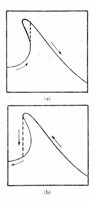
Fig. 2.9 The response of a non-linear softening spring system as the frequency of the driving waveform is (a) increased and (b) decreased. The theoretically predicted response is shown by the solid line, but as the driving frequency (abscissa) is changed, the response (ordinate) "jumps" upward or downwards (dotted line). The size of the response is therefore unstable and unpredictable over a certain band of frequencies.
