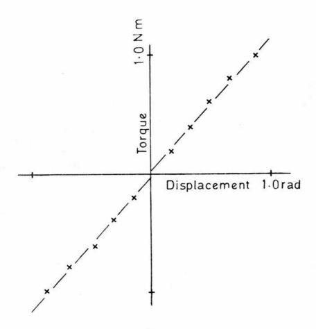
Fig. 3.34 Compliance of mechanical model. The compliance is linear and has a value of 1.25 N m rad<sup>-1</sup>. The compliance line does not, however, pass through the origin; 0.05 N m torque is required to produce a displacement. This is due to static friction in the motor (G9M4).
