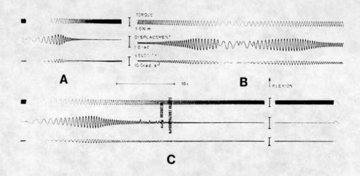
Fig. 3.7 Resonance produced by different types of sweep. At "A" resonance is produced by a "conventional" logarithmic sweep. At "B" a manually controlled decreasing and increasing frequency was employed. At "C" the range of frequencies swept is the same as at "A", but the sweep is linear rather than logarithmic. The resonant frequency is the same in each case (2.1 Hz). (Subject G.W.W. 45 m left wrist).
