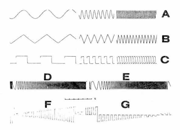
Fig. 2.5 Some typical waveforms:- (A) sine, (B) triangular, and (C) rectangular torques - max frequency 25 Hz, torque 1.0 N m, min frequency 0.1 Hz, torque 0 N m, (D) logarithmically and (E) linearly ramped sinusoidal torque; ramp length adjustable from 0 - 45 s, (F) biphasic rectangular torques, amplitude automatically increasing, and (G) monophasic rectangular torques - amplitude automatically increasing and decreasing - no. of steps 2 - 256, torque 0 - 1.0 N m.
