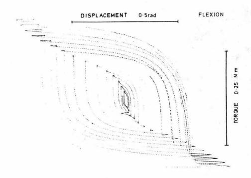
Fig. 3.30 Composite compliance curve of the wrist. Torque vs displacement has been plotted using a X-Y recorder. One point is plotted for each torque reversal. This gives a complete picture of the non-linear stiffness of the wrist; the stiff region is obvious, as is the region of increased compliance and finally the region of increasing stiffness for the largest torques. Overshoots are seen with the largest torque pulses.
