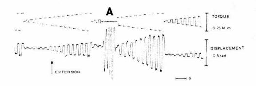
"Thixotropy" in cooled muscle. This record was obtained from a wrist following immersion of the forearm in water at 7°C for 20 mins. Originally the compliance is low (about 30% of the control value). At "A" the subject made 4 flexion/extension movements of the wrist and as a result the compliance during the next cycle of ramped rectangular torques was increased considerably.
