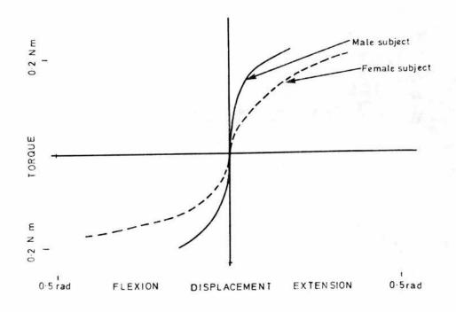
Fig. 3.31 Compliance of a male and female subject, traced from composite compliance curves. The displacement of the female subject is greater at all levels of torque and the size of the stiff region is smaller.
