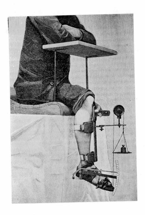
Fig. 1.2 The earliest machine for the measurement of muscle tone in man; the "myotonomètre" of Mosso (1896).
