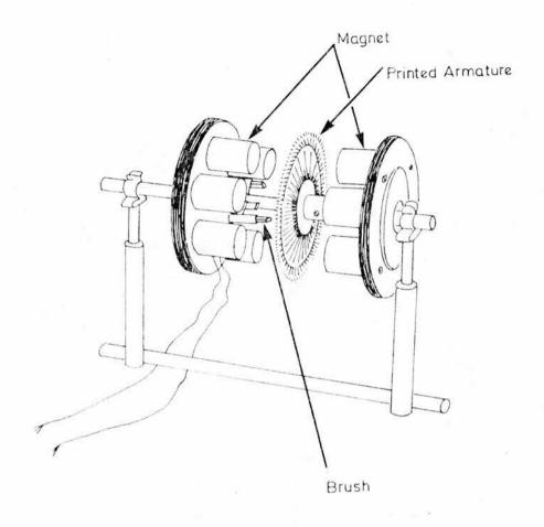
$\underline{\text{Fig. 2.3}}$  An "exploded" view of the main components of the G6M4 printed armsture motor used in the investigations.
