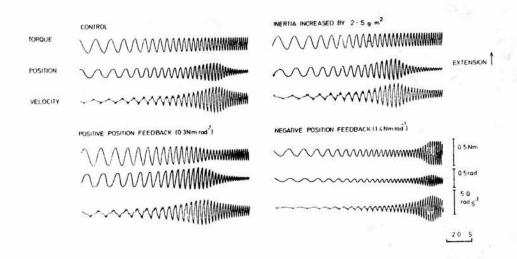
Fig. 3.19 Resonance of the wrist with the addition and subtraction of stiffness, and the addition of inertia. The resonant frequency initially is 2.8 Hz. Added inertia and positive position feedback slow this to 2.2 Hz and 2.4 Hz respectively. Negative position feedback increases resonant frequency to 4.7 Hz. (Subject M.L. 26 m right wrist).
