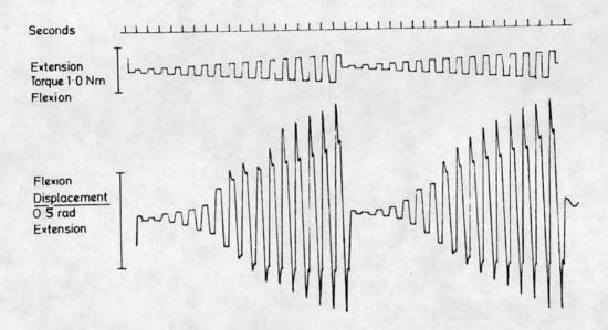
Fig. 3.29 Ramped rectangular torques. A linearly increasing series of torque pulses is applied to the relaxed wrist. The compliance is non-linear; the first 4 or 5 torque impulses produce a disproportionally small displacement. The compliance then increases rapidly, and finally begins to decrease gradually. The system is evidently heavily damped for small displacements; overshoots are not seen when the torque is small. (Subject C.E.H. 22 f left wrist).
