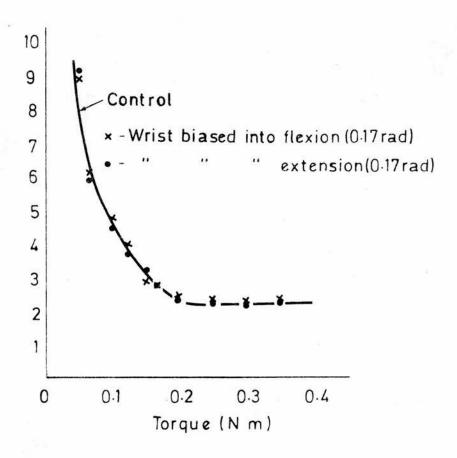
Fig. 3.18 Bias experiment; torque vs resonant frequency. The control curve was plotted from measurements of resonant frequency at 10 torque levels; movement occurred about the natural resting position of the wrist. The resonant frequency of the wrist with these same torques is shown following a bias of  $20^{\circ}$  (0.34 rad) into flexion and extension. The pattern of non-linearity is not changed by this manoeuvre.
