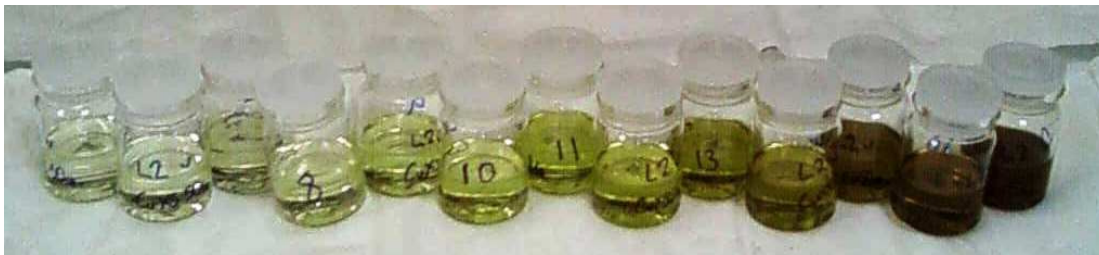
Figure 2.23: Photograph of the organic phases of the extraction of copper(II) by L2 , showing an ideal range of copper loading from pH 0-3.5.
