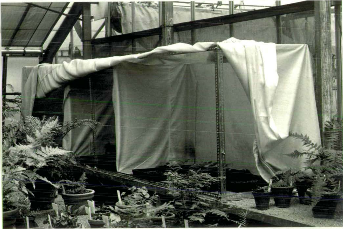
Figure 10.1. The shade frame. This was assembled from dexion in the greenhouse at the Royal Botanic Garden, Edinburgh, and provided three levels of shading. The shade cloth used was close weave standard thickness.
