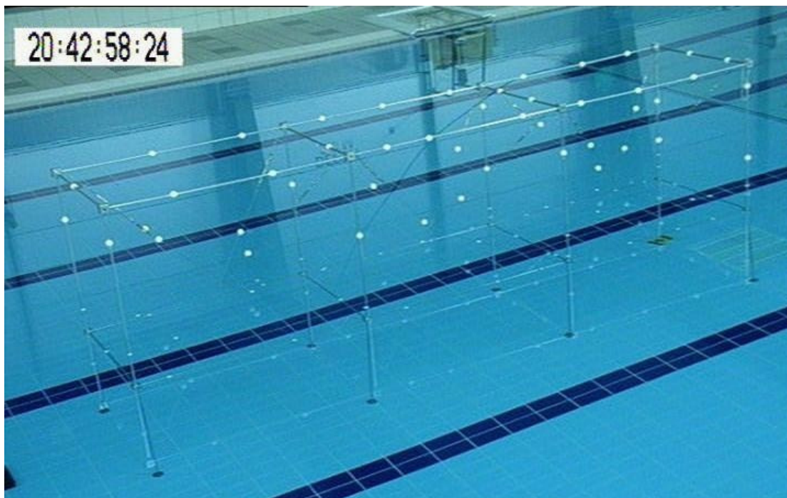
Figure 3.9: An above water view of the calibration frame from camera 5 perspective.
