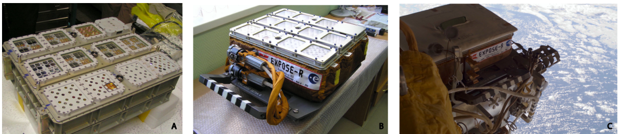
Figure 4.2 The EXPOSE-R facility A) During sample integration B) Awaiting launch C) Outside of the International Space Station (source: NASA)
