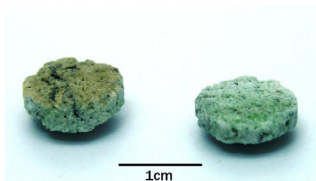
Fig. 3. Image showing colour change in UV-exposed rocks (left) compared to rock kept dark in LEO (right).
