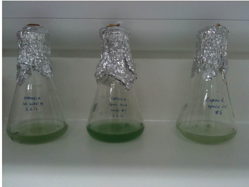
Figure 4.5 Growth of Chroococcidiopsis in BG-11 medium inoculated with rock discs from all conditions. Left to right: stored in lab, dark in low Earth orbit and UV exposed in low Earth orbit. Growth is observed in all flasks. Picture taken after 2.5 months of incubation
