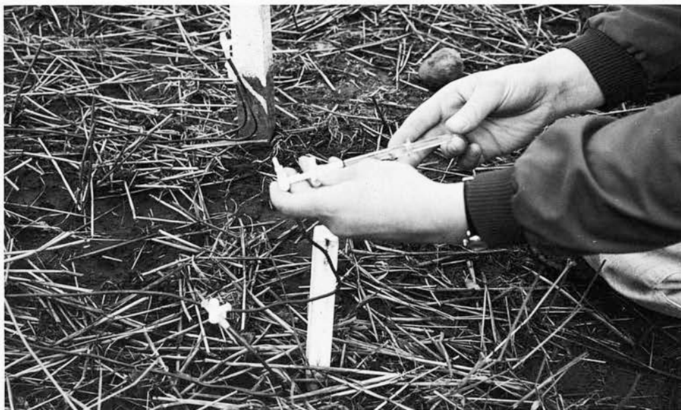
Sampling from a probe: The tap of a syringe was fitted into the tap of a sampling point and the two held together.
