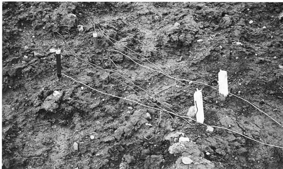
Soil atmosphere sampling probes at a depth of 15 cm and 30 cm sited in a ploughed plot. These probes have thermistors attached.
