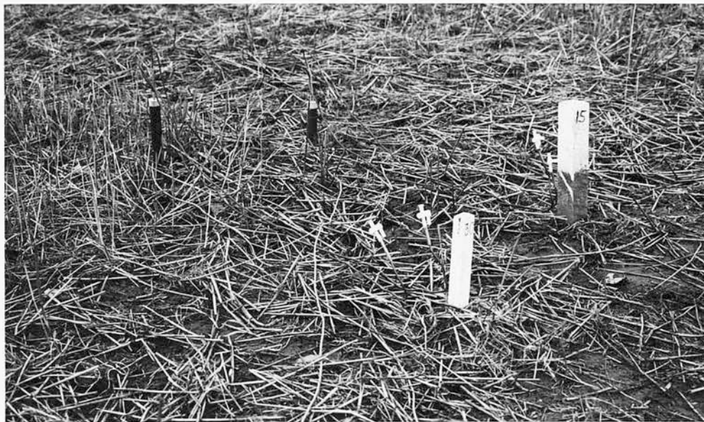
Soil atmosphere sampling probes at a depth of 15 cm and 30 cm sited in a no-tillage plot.
