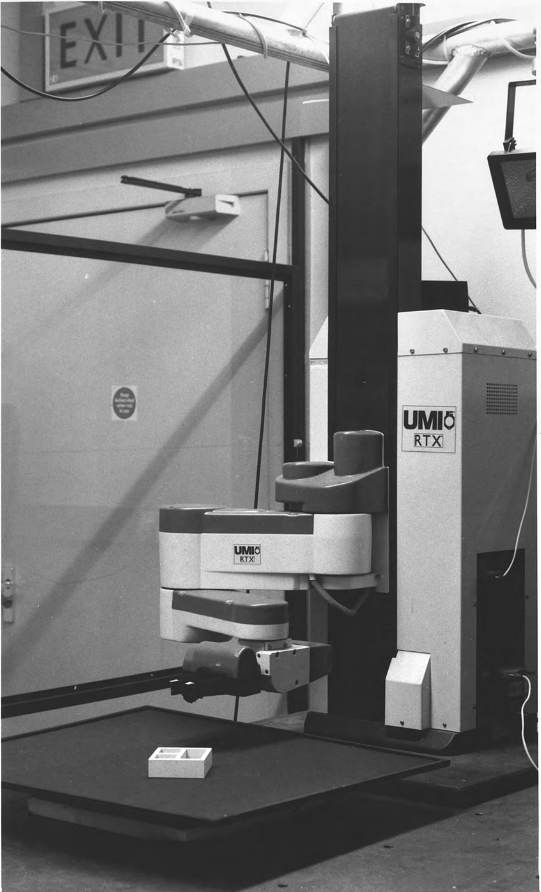
Figure 4.1: RTX robot and Force Table
