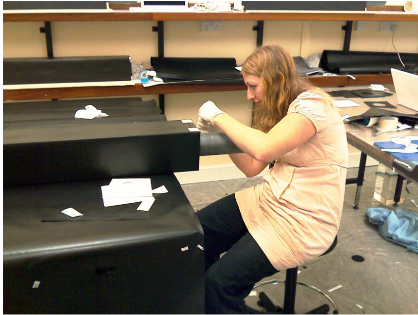
Figure 4.11: Wrapping the scintillator sections. Here a scintillator block is undergoing wrapping with a black light tight sheet. This was performed after the PMT cap had been glued and after the block had been wrapped with PTFE.
