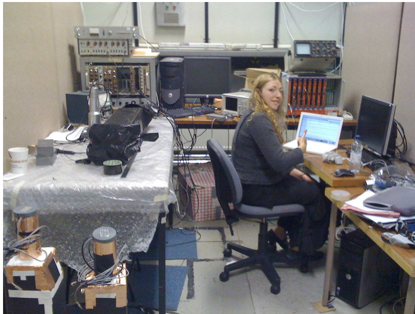
Figure 5.3: The experimental set-up at the University of Edinburgh. To the left of the figure is a scintillator block within its light tight wrapping undergoing testing. At the back of the figure are the electronics and MCA readout (Maestro).
