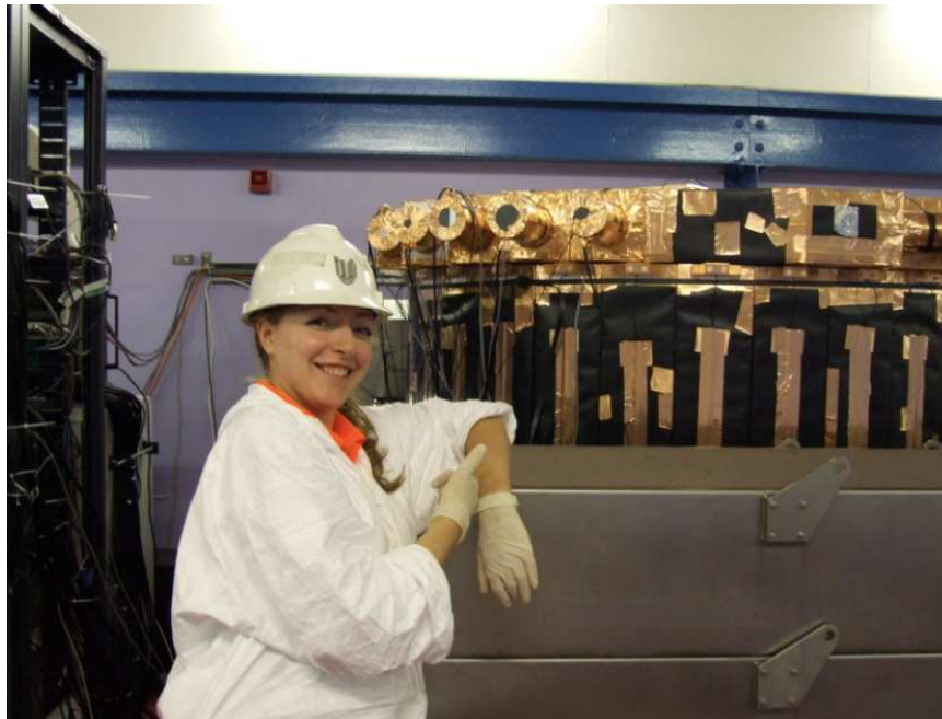
Figure 4.15: The veto partially shielded with lead. The entire structure of the veto is surrounded by lead.
