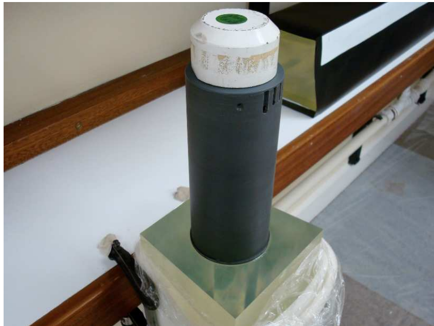
Figure 4.9: The PMT caps were glued onto the scintillator sections. The caps serve two purposes, firstly to protect the PMT from external light sources and secondly to hold the PMT into position.
