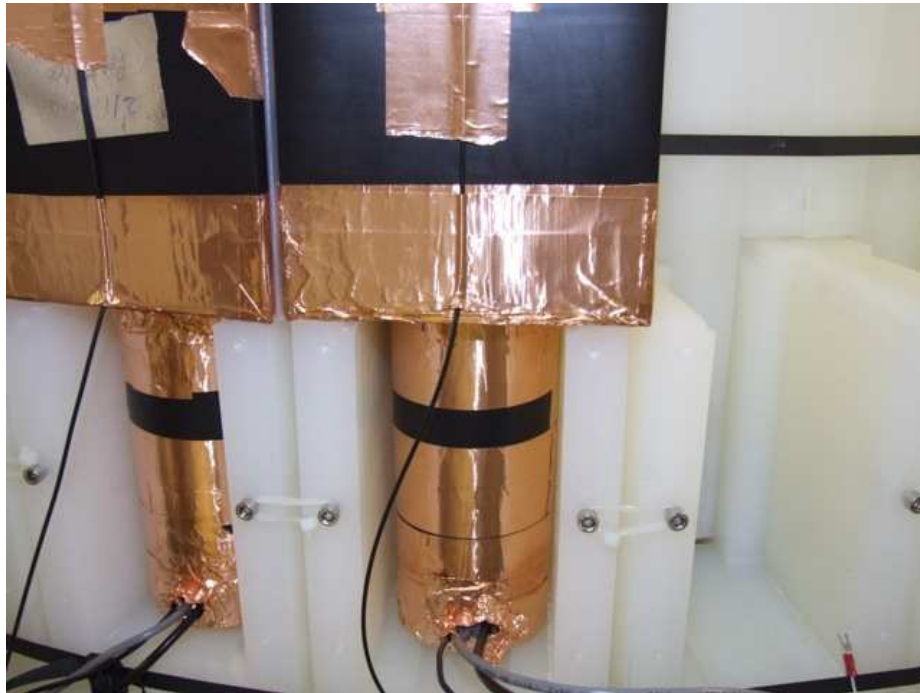
Figure 4.4: Positioning of the veto PMTs in the base of the passive shielding. The scintillator section rests on top with room provided for its corresponding PMT. The PMT is sealed using a separate polypropylene back piece (not shown).
