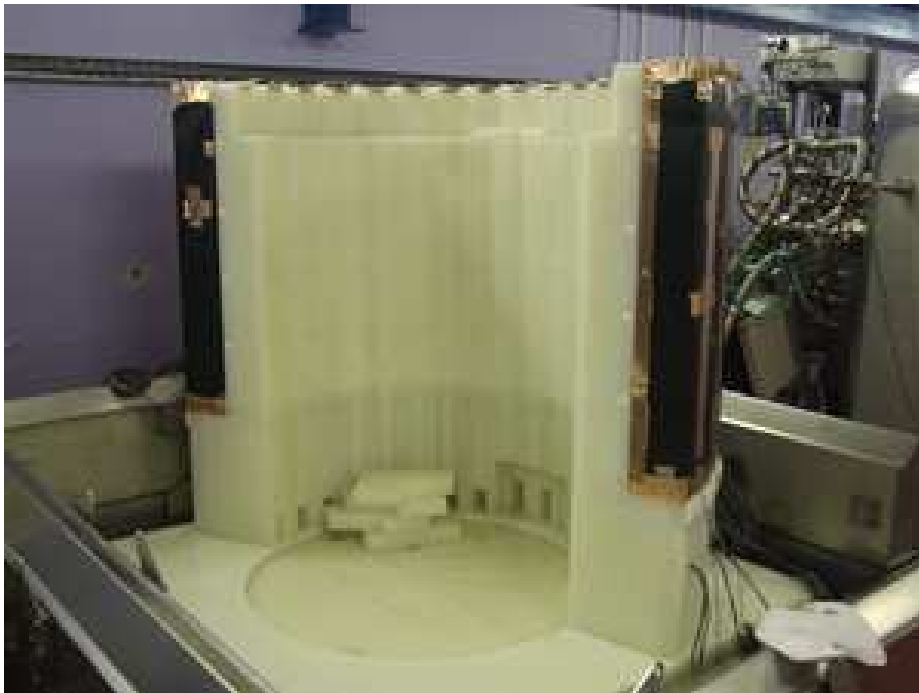
Figure 4.1: The active (black) and passive (white) components of the veto are displayed in situ. The ZEPLIN-III detector would sit at the centre of the veto where the circular cut-out section can be observed in the shielding base. Only 50% of the walls are shown in the figure, the entire veto system resembles a barrel type structure which surrounds the entire ZEPLIN-III vessel. The roof sections are also not shown.
