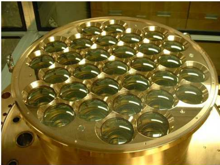
Figure 3.7: The ZEPLIN-III PMT array. The array include 31 PMTs positioned within the ZEPLIN-III target vessel and immersed in liquid Xe.
