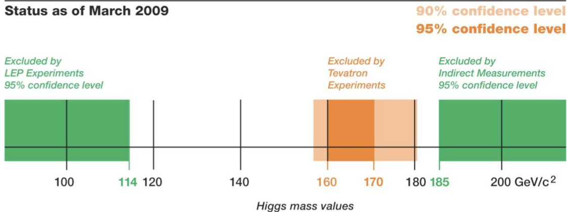
Figure 1.16: Current experimental constraints on the Higgs mass from indirect searches, the Tevatron and LEP experiment at CERN indicate a mass within the range \sim 114 - 160 GeV/ c^2 . The Large Hadron Collider will probe this region from 2010 with the aim of detecting the Higgs Boson [60].
