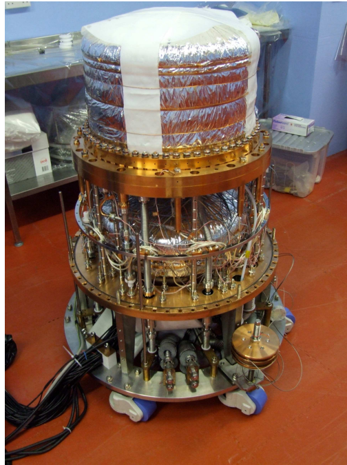
Figure 3.6: The internal structure of the ZEPLIN-III device. The top dome object is the target vessel. Below this is LN 2 reservoir.
