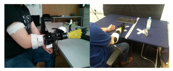
Figure 3.10: Socket fitting for real-time experiment. Customised sockets were built for ablebodied subjects (left) and the amputee participant (right).
