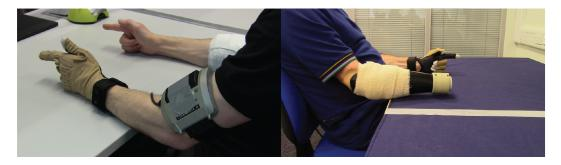
Figure 8.4: Bilateral mirrored movement training. Two participants, an able-bodied (left) and an amputee (right), shown during training data collection. Muscle activity was recorded from the participants' right forearm (i.e. the phantom limb for amputees), whereas hand kinematic data were recorded from the participants' left hand with an 18-DOF data glove.
