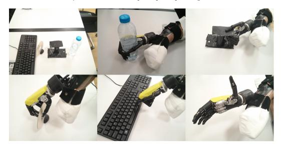
Figure 3.11: Real-time control pick and place experiment. Participants were instructed to use a prosthetic hand to grasp, relocate, and release three objects and finally press the "space" key on a computer keyboard. Five grip types were used: power/cylindrical (water bottle), lateral (credit card simulator), tripod (CD), index finger pointer (computer keyboard), and hand opening.
