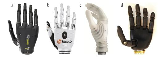
Figure 2.3: Modern commercial prosthetic hands. (a) Touch Bionics i-limb<sup>™</sup> (Touch Bionics, Inc., 2003); (b) Ottobock bebionic (Ottobock, Inc., 1919); (c) Ottobock Michelangelo (Ottobock, Inc., 1919); (d) Vincent Evolution 2 (Vincent Systems, GmbH, 2013). All photographs have been provided and are used with permission from the respective manufacturers.
