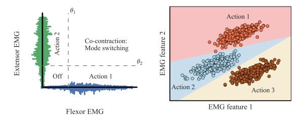
Figure 2.5: Mode switching vs. classification-based myoelectric control. (Left column) an example of amplitude-based mode switching myoelectric control paradigm. Based on a figure by Parker, Englehart, and Hudgins (2006). (Right column) a qualitative illustration of a three-class myoelectric control scheme using a linear classifier (LDA) and two EMG features.
