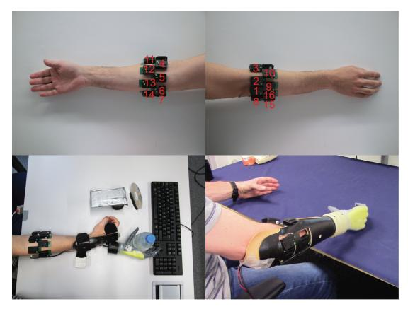
Figure 5.1: Experimental setup. Sixteen sensors were placed on the subjects' forearm below the elbow in two rows of eight equally-spaced sensors (top row). Custom built sockets were used to accommodate the robo-limb prosthetic hand for able-bodied (bottom left) and amputee (bottom right) subjects.
