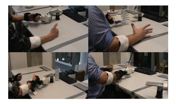
Figure 8.7: Pick and place task. Two able-bodied participants shown while they use the prosthetic hand to grasp, relocate, and release the objects used in the experiments. (Top row) EMG control mode; (bottom row) data glove control mode.
