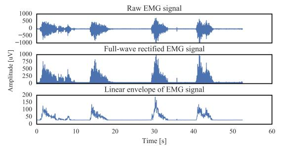
Figure 2.4: An example of EMG signal linear envelope extraction. The raw EMG signal (top panel) is firstly full-wave rectified (middle panel) and subsequently smoothed via low-pass filtering (bottom panel).
