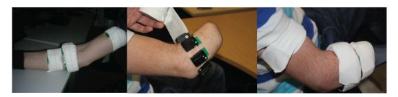
Figure 3.4: Sensor placement. Eight EMG-IMU sensors were equally spaced around the participants' forearm (3 cm below the elbow), two targeted the extensor digitorum communis and flexor digitorum superficialis muscles, and two were placed on the biceps and triceps muscles. Elastic bandage was used to keep the sensor positions fixed. Sensor placement shown for an able-bodied (left) and an amputee subject (centre, right).
