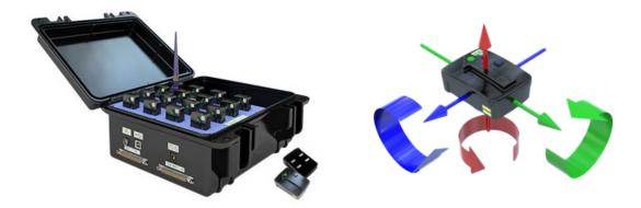
Figure A.1: Delsys® Trigno<sup>TM</sup> IM system. (Left) the full platform including the base station and sensors; (right) a single Trigno IM sensor incorporating an EMG electrode and an IMU. The IMU comprises three tri-axial components, that is, an accelerometer, a gyroscope, and a magnetometer providing 3D measurements of acceleration, angular velocity, and magnetic field, respectively. Photographs provided by and used with permission from Delsys, Inc. (Delsys, Inc., 1993).
