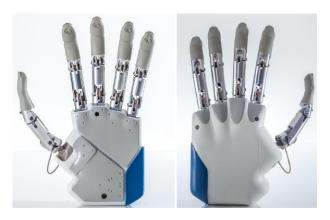
Figure A.3: Prensilia IH2 Azzurra hand (left-hand model). Palmar and dorsal views of the hand are shown. Photographs provided by and used with permission from Prensilia S.R.L. (Prensilia, S.R.L., 2009).
