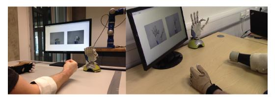
Figure 8.6: Posture matching task. An able-bodied (left) and an amputee participant (right) shown while they modulate their muscle activity to drive the robotic hand into the desired posture. The target postures for the shown trials were full cylindrical grip and half index flexion, respectively.
