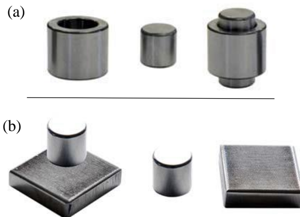
Fig 2.8 Devices used within a BAM hammer (BFH-12) a Impact device 1, consisting
