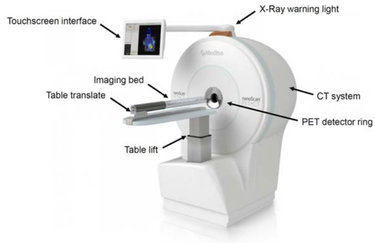
Figure 2.4: The nanoScan PET/CT camera. The imaging bed was accurately positioned using the table translate and table lift. The touchscreen interface on the PET/CT scanner or the acquisition workstation were used to move the scanner bed, or to monitor of the vital functions of the rats during in vivo experiments (Image from Mediso, 2015).
