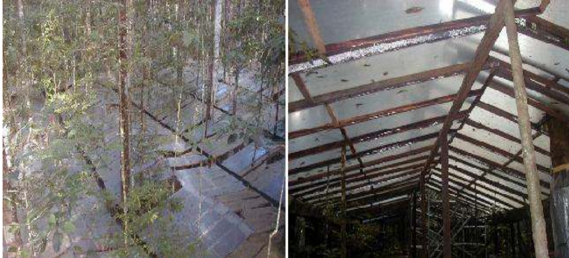
Figure 2. View (a) above and (b) below the plastic panels on the OX dry plot.
