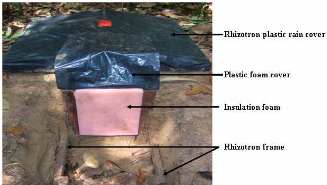
Figure 2. An installed rhizotron. Note insulation foam in place covering the observation screen, a plastic cover (folded over) which usually protects the screen from light and rainfall. The larger plastic rain cover is set behind the rhizotron.
