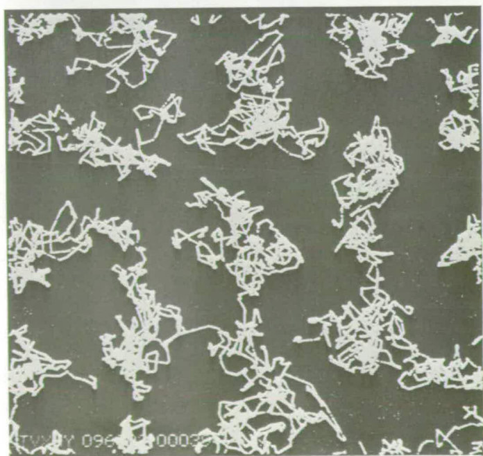
Fig. 1. Trajectories of hard-sphere particles are displayed on a cathode ray tube hooked directly to a computer. Top shows solid state, bottom liquid. Reprinted from Ref. (8), p. 124, by courtesy of Scientific American, Inc.
