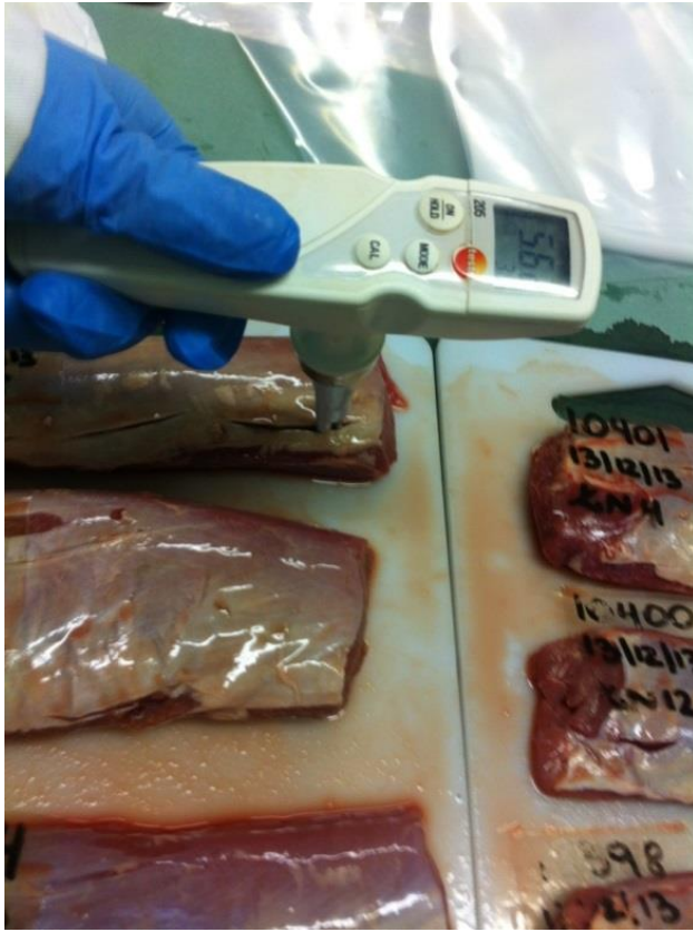
Figure 2 Measurement of ultimate pH and temperature of loins by Hannah testo-205 probe in three sections across the loin.
