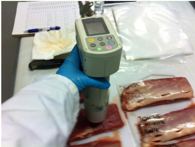
Figure 3 Measurement of Lightness ( L^* ), redness ( a^* ) and yellowness ( b^* ) of meat by Konica Minolta 410 chromometer.
