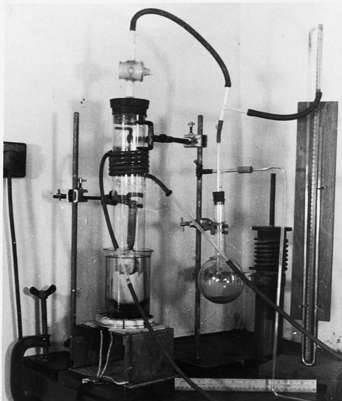
PLATE III. Fig. 16. Arrangement for Vacuum Impregnation.
