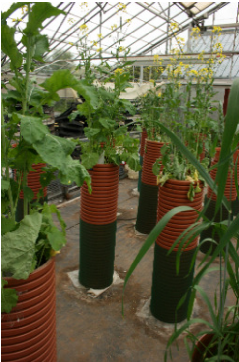
Photo 1 The lysimeters with oilseed rape and wheat plants at the day of harvest. The green mesh shading the mini crops during growth was slid down.
