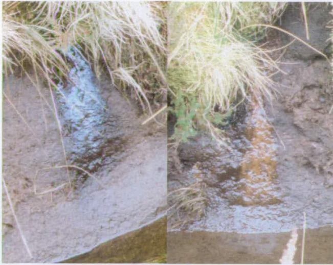
Figure 4.43: Drainage ditch metallic staining (a-black stain; b-orange stain)
