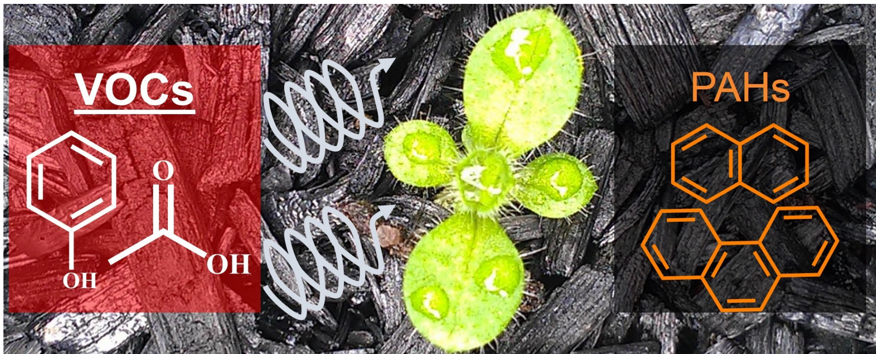
Figure 9.1: Graphical abstract of Chapter 9. In biochars contaminated with pyrolysis vapours, both, VOCs and PAHs, were detected in concentrations high enough to cause phytotoxic effects. However, it was concluded that with a high probability VOCs were responsible for previously observed plant inhibitions caused by these biochars. This was attributed to the higher mobility and phytotoxicity of VOCs compared to PAHs.
