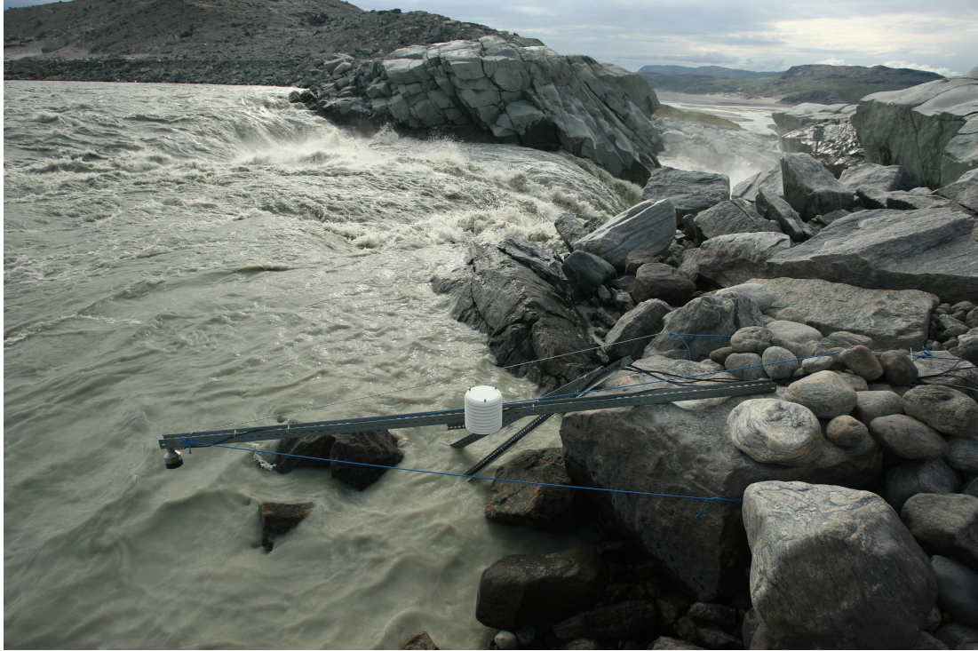
Figure 3.9: Hydrological monitoring station in the proglacial stream. Pressure transducers, turbidity meters and an electrical conductivity meter are mounted on a support structure which is fixed to bedrock and are submerged at a fixed height. A UDG is also suspended above to channel to provide a secondary record of river stage.
