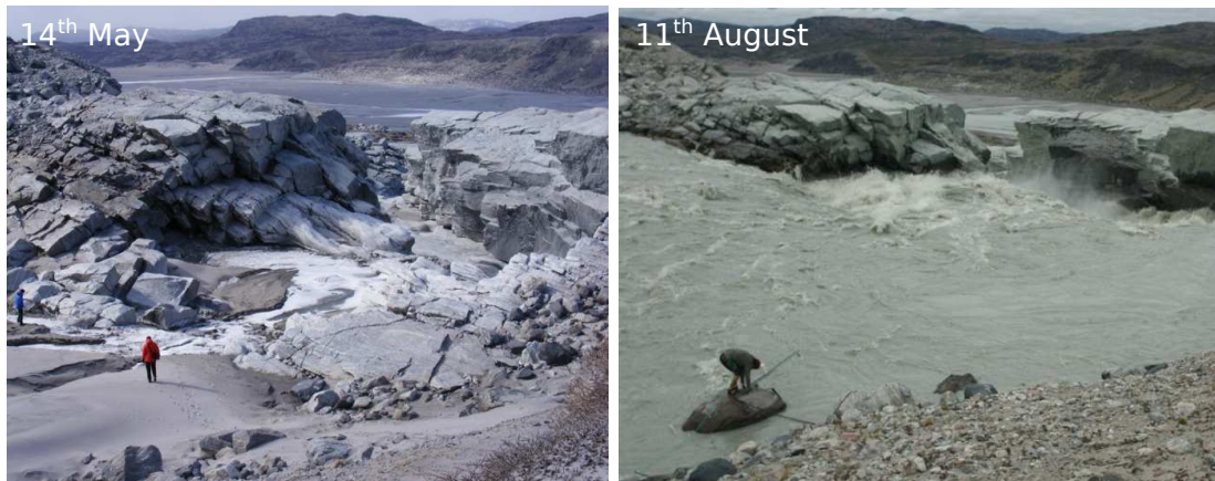
Figure 3.8: River cross-section where hydrological measurements were made (dates in the photographs are from 2009). At the start of the melt season the river bed is empty and discharge grows to several hundred \text{m}^3 \text{s}^{-1} by late summer. The cross-section is located at the top of a large waterfall approximately 2 km from the glacier snout (see Figure 3.3).
