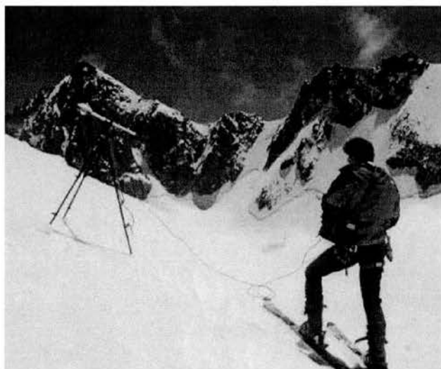
Figure 5.11. Albedometer setting. The white oval, above and left the camera tripod is the albedometer, made up of two Kipp & Zonen opposed pyranometers. The output is read in two voltmeters connected at the extreme of the cable, hold by the skier-operator in the image.
