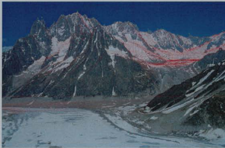
Figure 5.5. Super imposition of the perspective projection of a DEM of the Mer de Glace glacier (Figure 5.4) over a photograph of the area. Red dots are the perspective projections of the original DEM grid cells, green dots are ground control points. The photograph is taken from the Refuge du Requin looking east-northeast.
