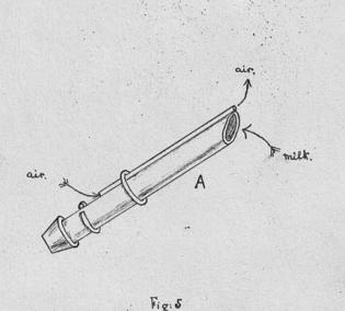
Instead of fixing on a teat a "Galactophore"(Fig. 5) may be inserted through the hole in the stopper.
