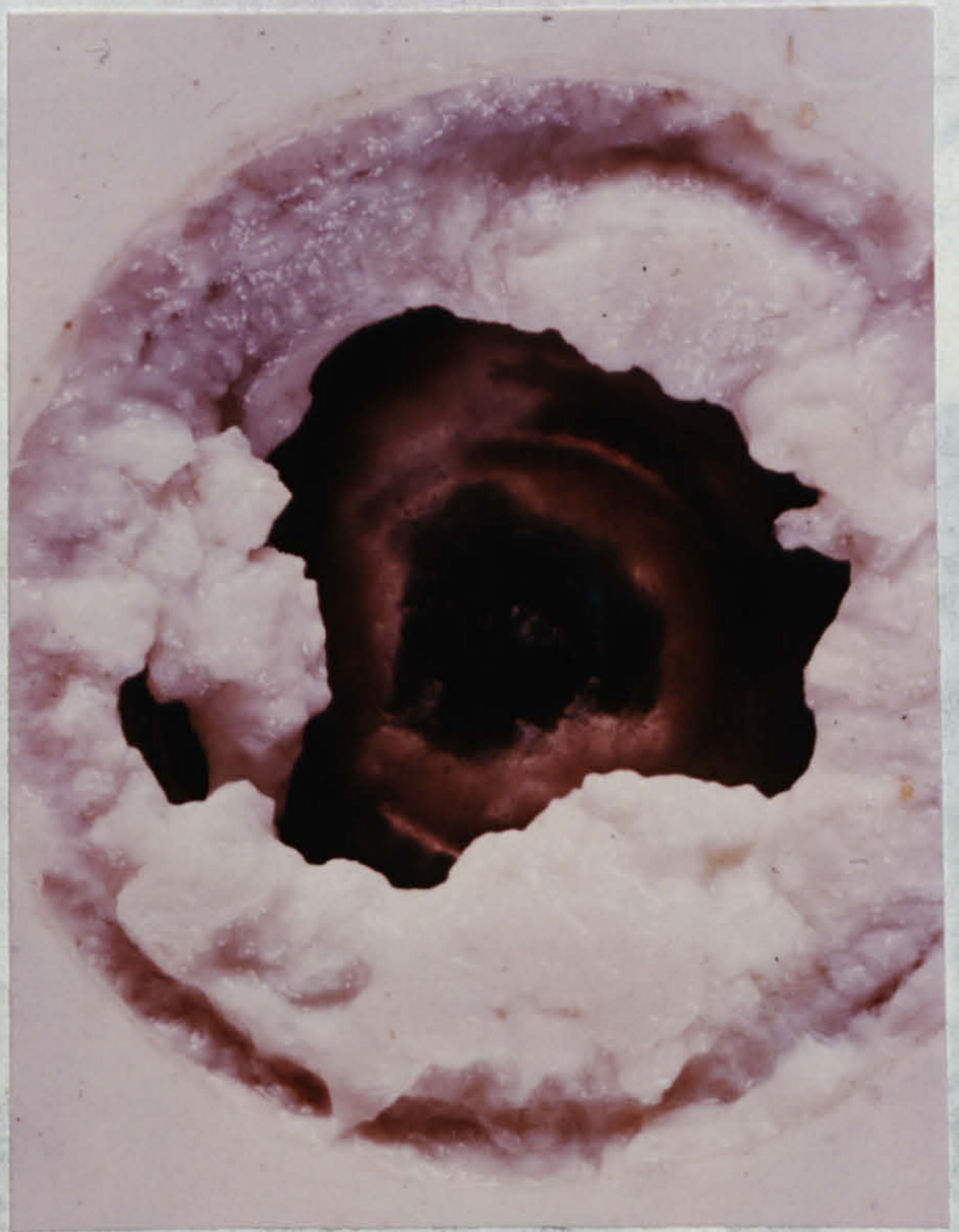
Fig 85. Milk. Starr-Edwards Aortic Upstream. 43°C. 0.6% CaCl 2 & rennet. 1.7L/min milk. After 10 Mins.
