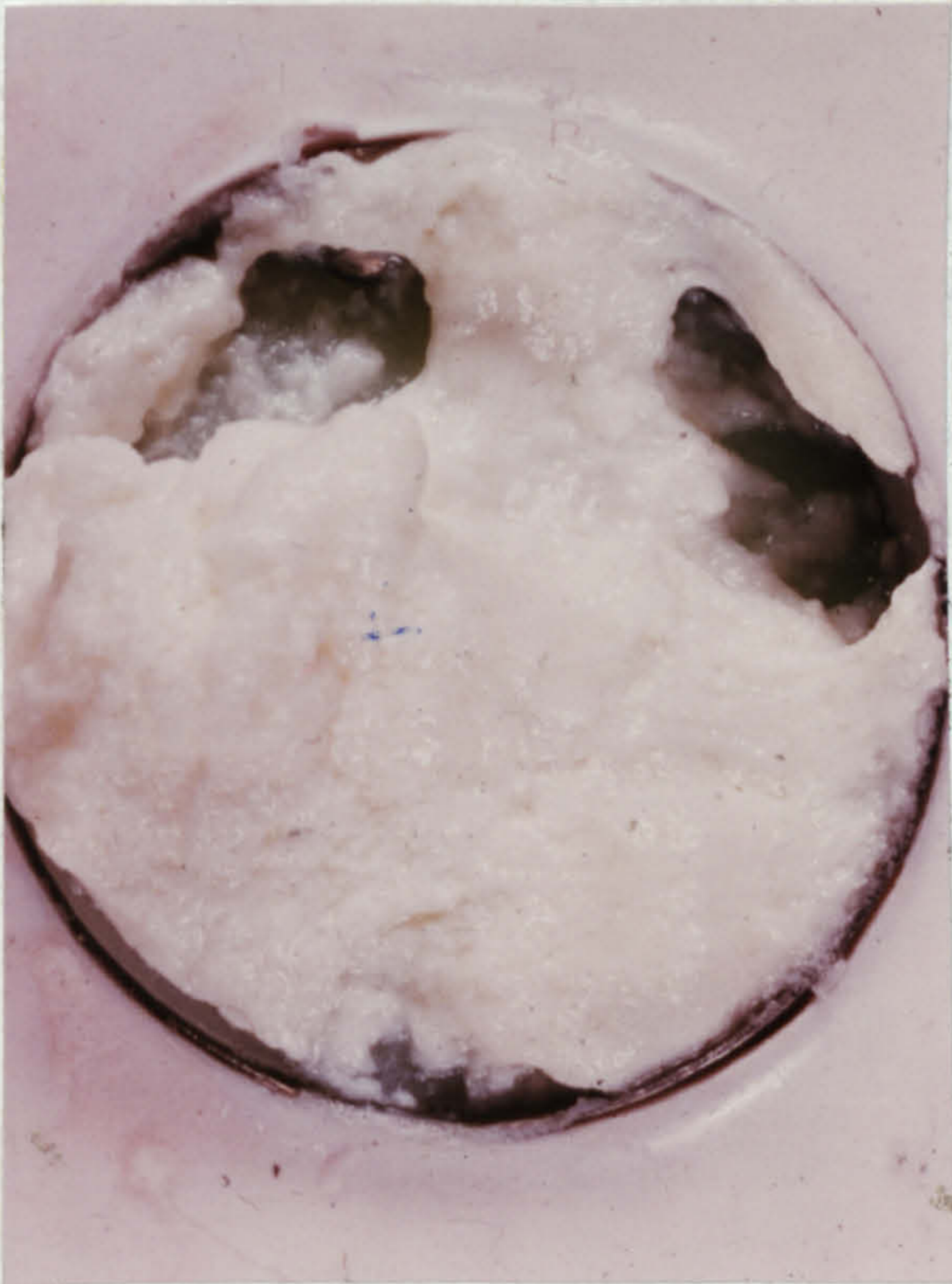
Fig 149. Flat Disc Mitral Downstream 43°C. 2L/min milk
