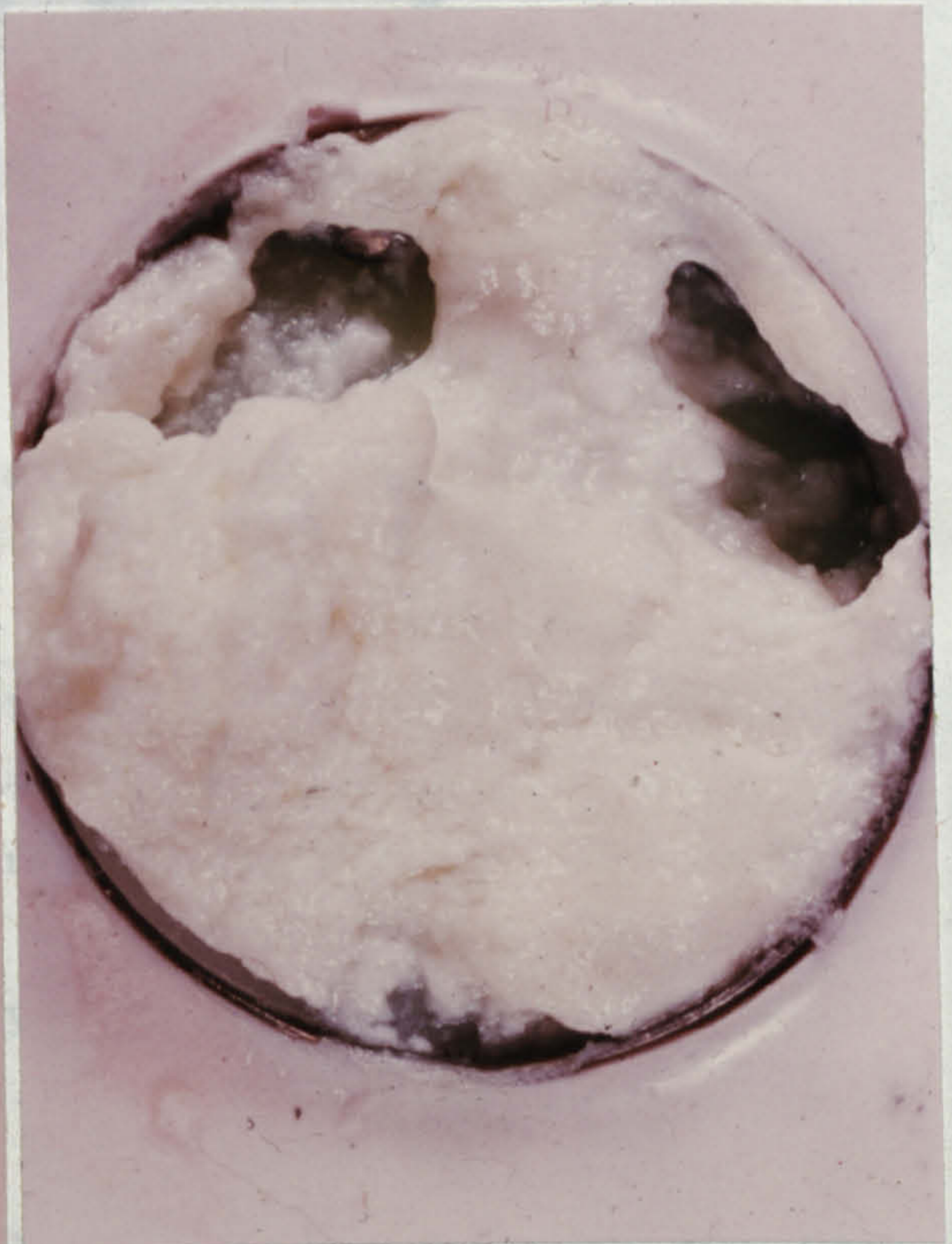
Fig 137. Flat Disc Mitral Downstream 43°C. 0.6% CaCl 2 and rennet. 1.7L/min milk. Pulse 50
