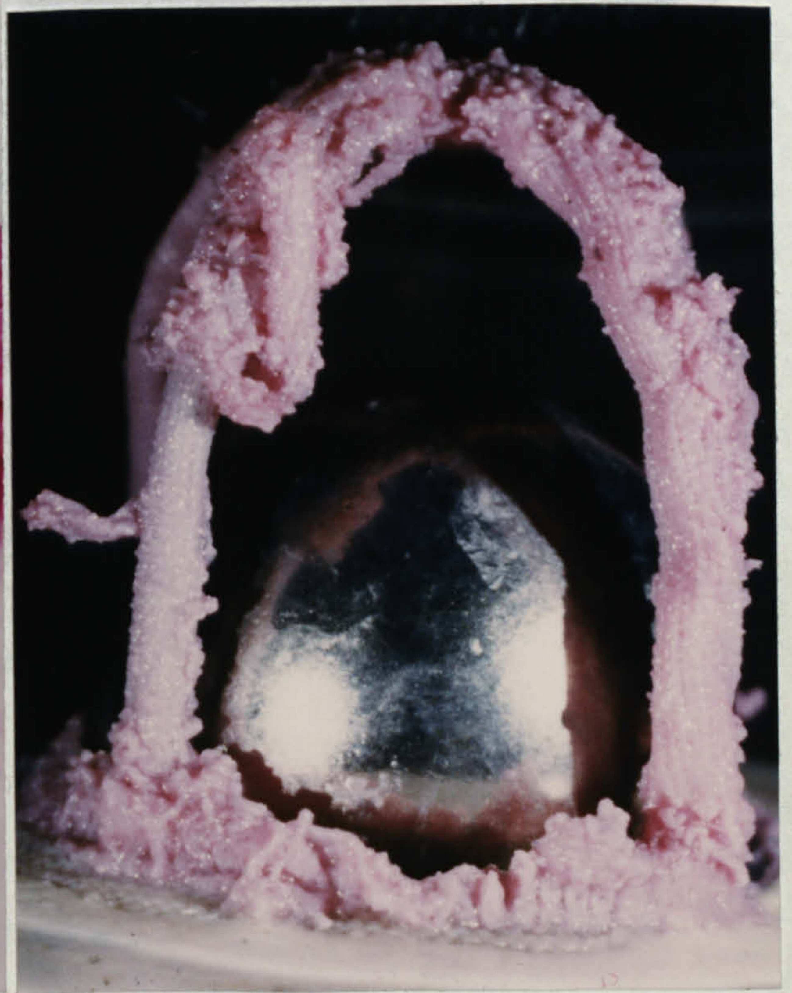
Fig 135. Starr-Edwards Aortic Upstream 38°C. 3L/min
