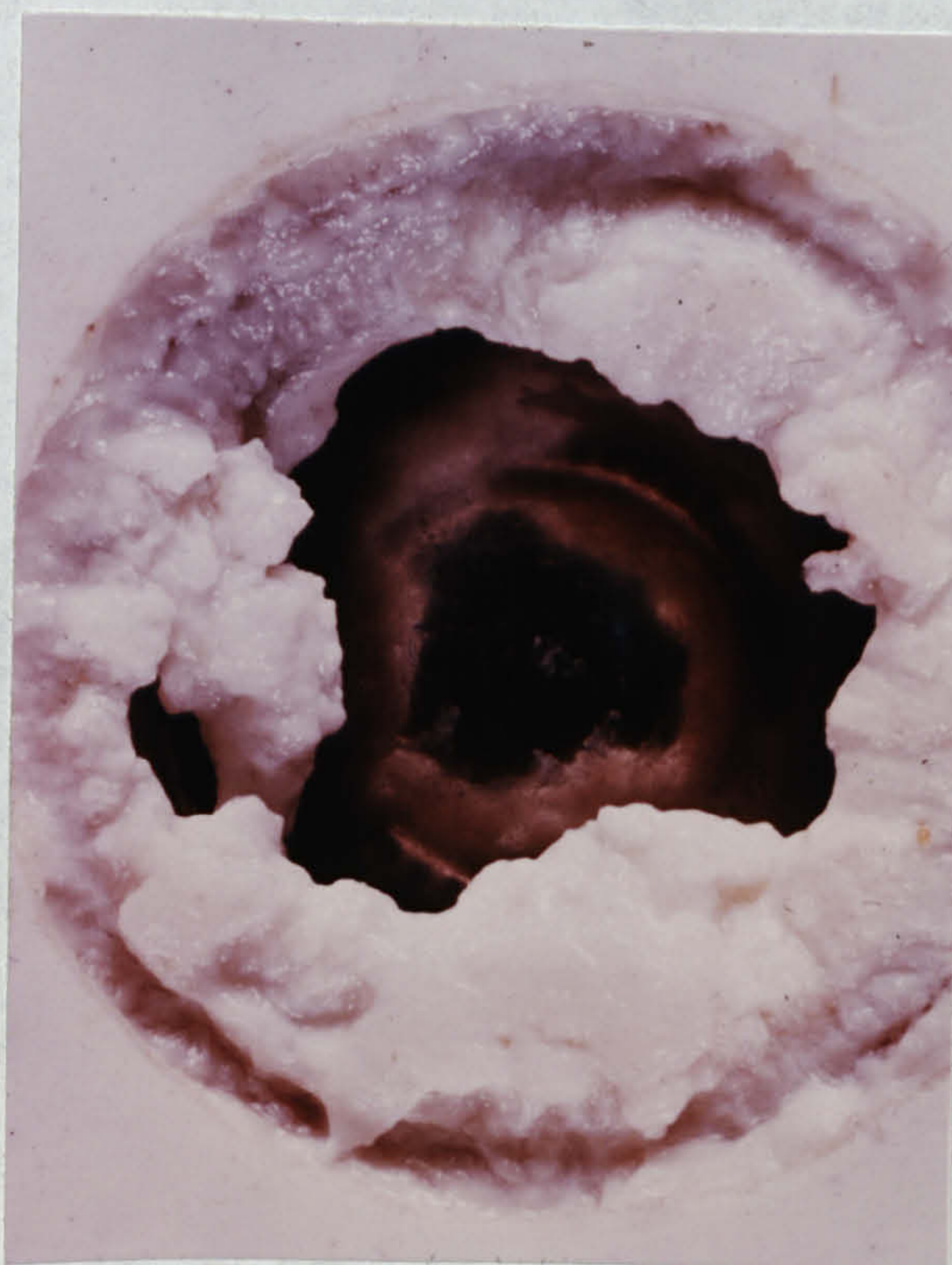
Fig 50. Starr-Edwards Aortic Upstream. 43°C. 0.6% CaCl 2 and rennet. 1.7L/min milk. Pulse 50. Run Duration 10 mins.
