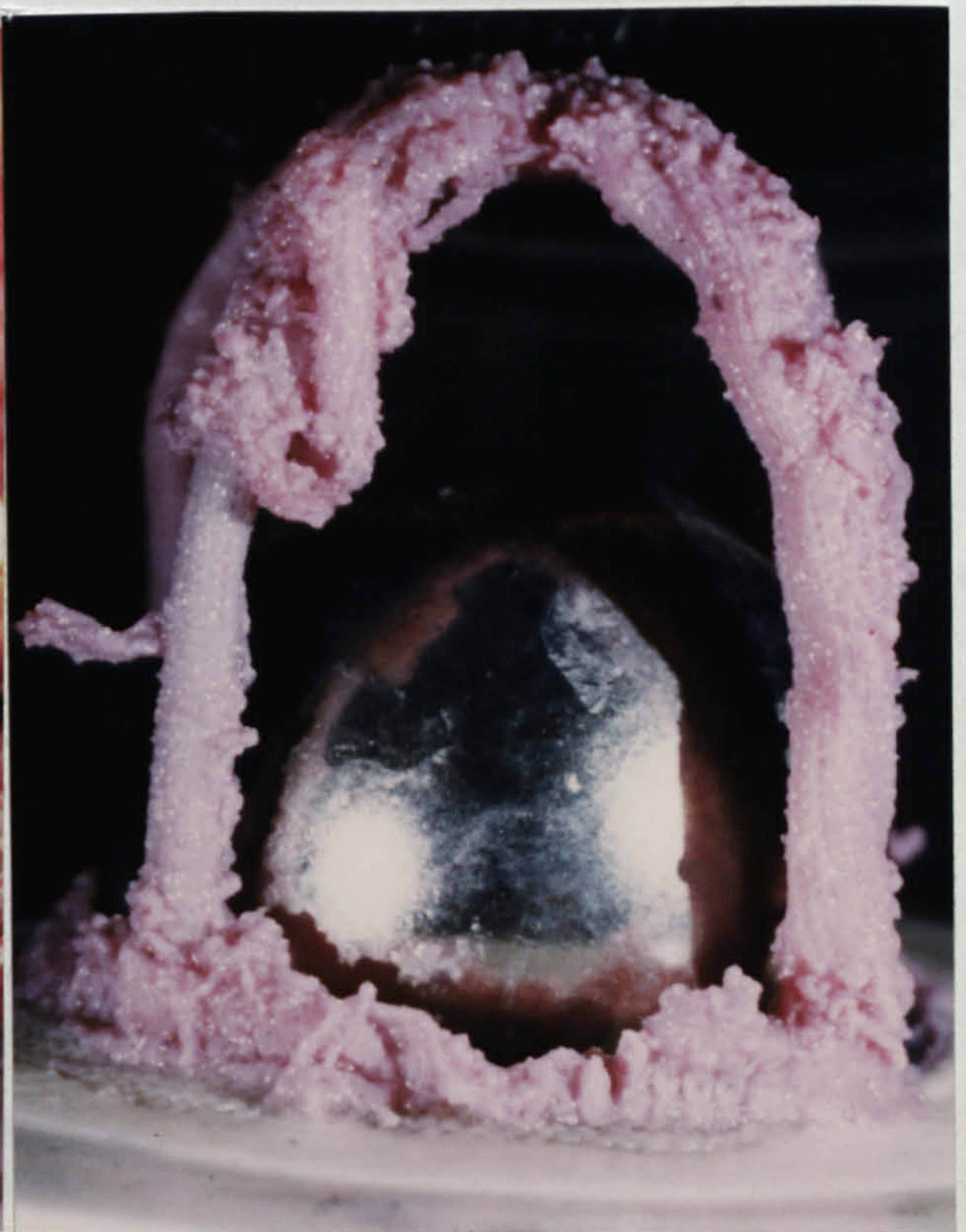
Fig 89. Milk. Starr-Edwards Mitral Downstream. 38°C. 3L/min milk.
