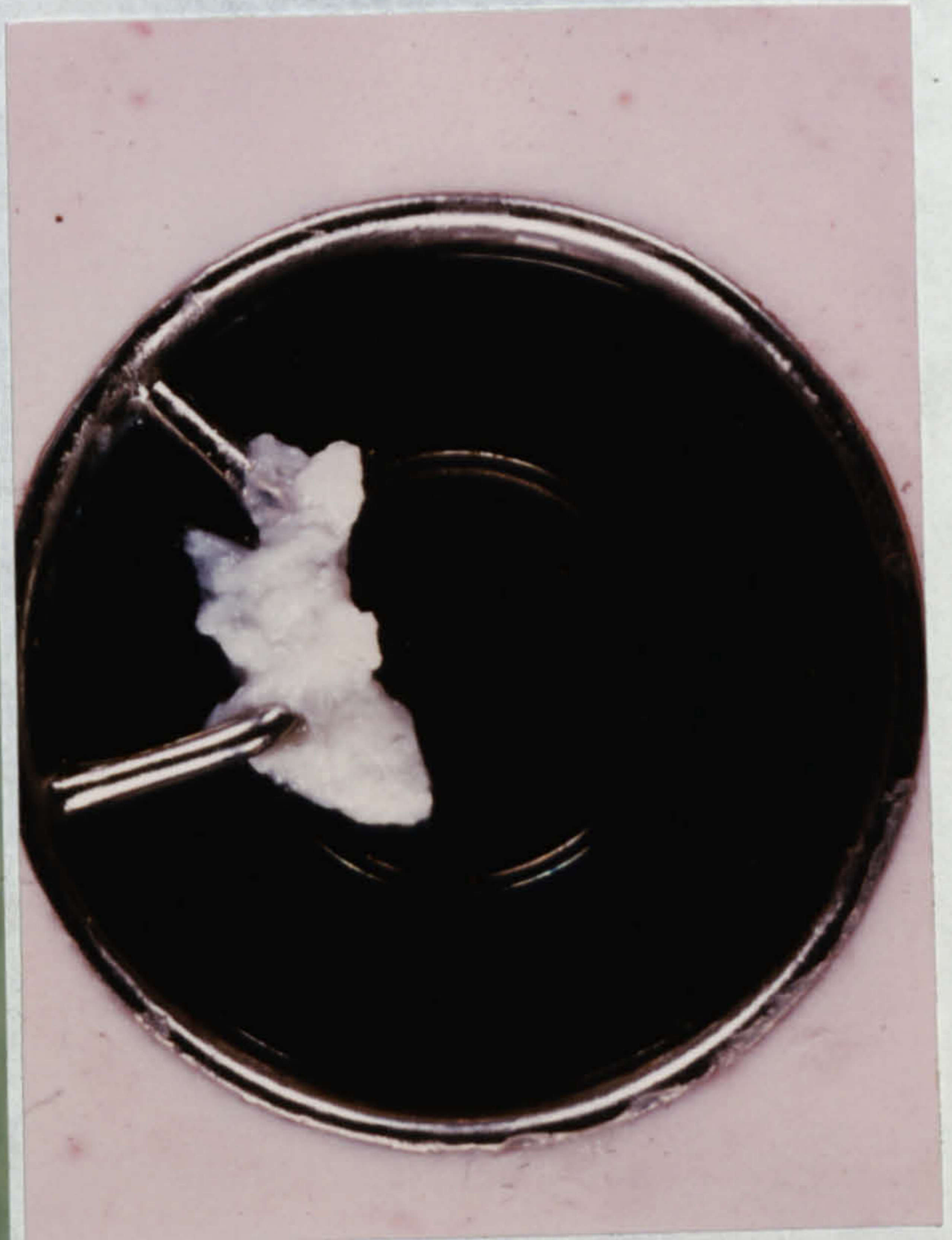
Fig 74. Milk. Bjork-Shiley Aortic Downstream. 40°C. 0.6% CaCl 2 & rennet. 2L/min milk. Albumen Coated.
