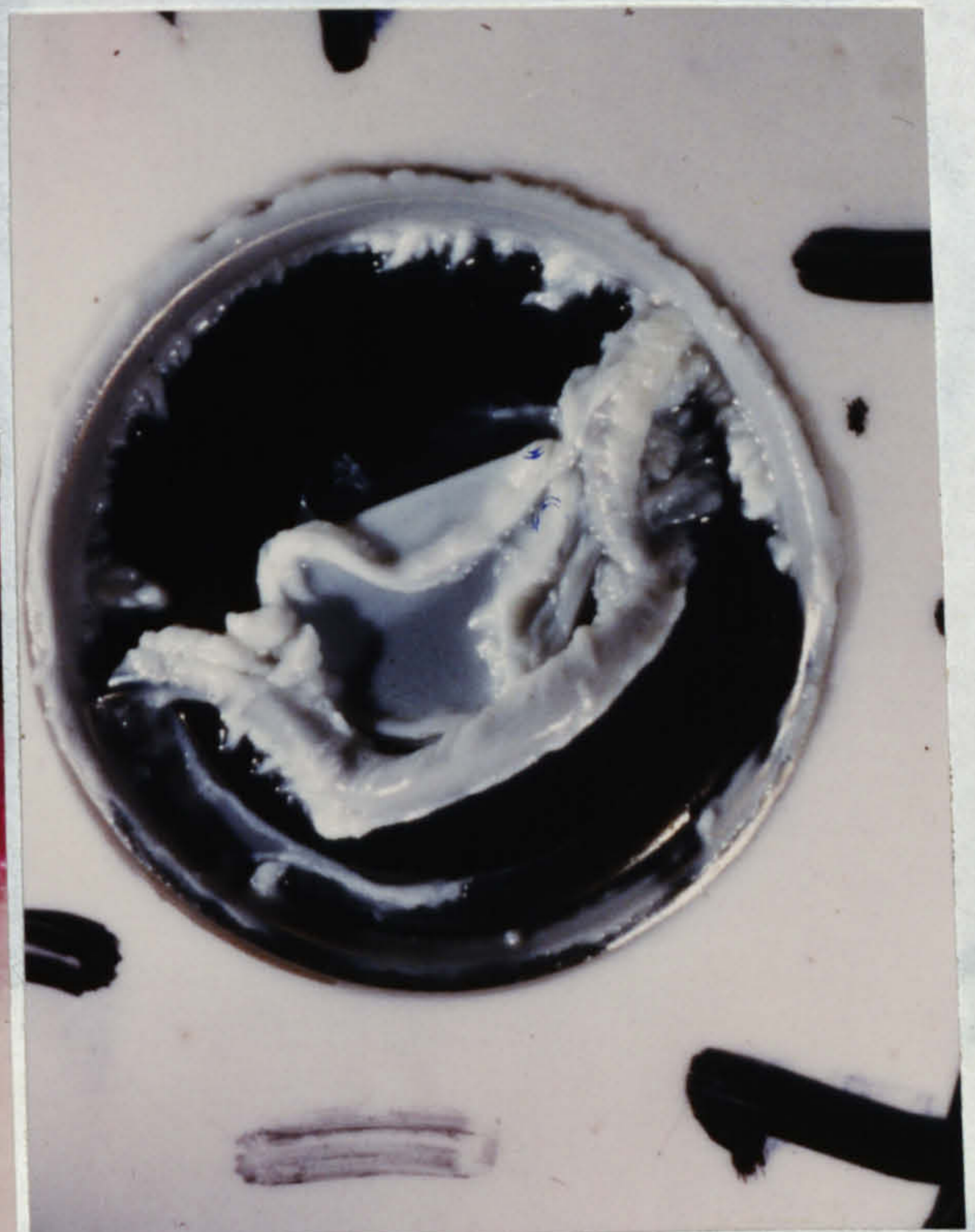
Fig 125. Bjork-Shiley Upstream 40°C. 3L/min milk
