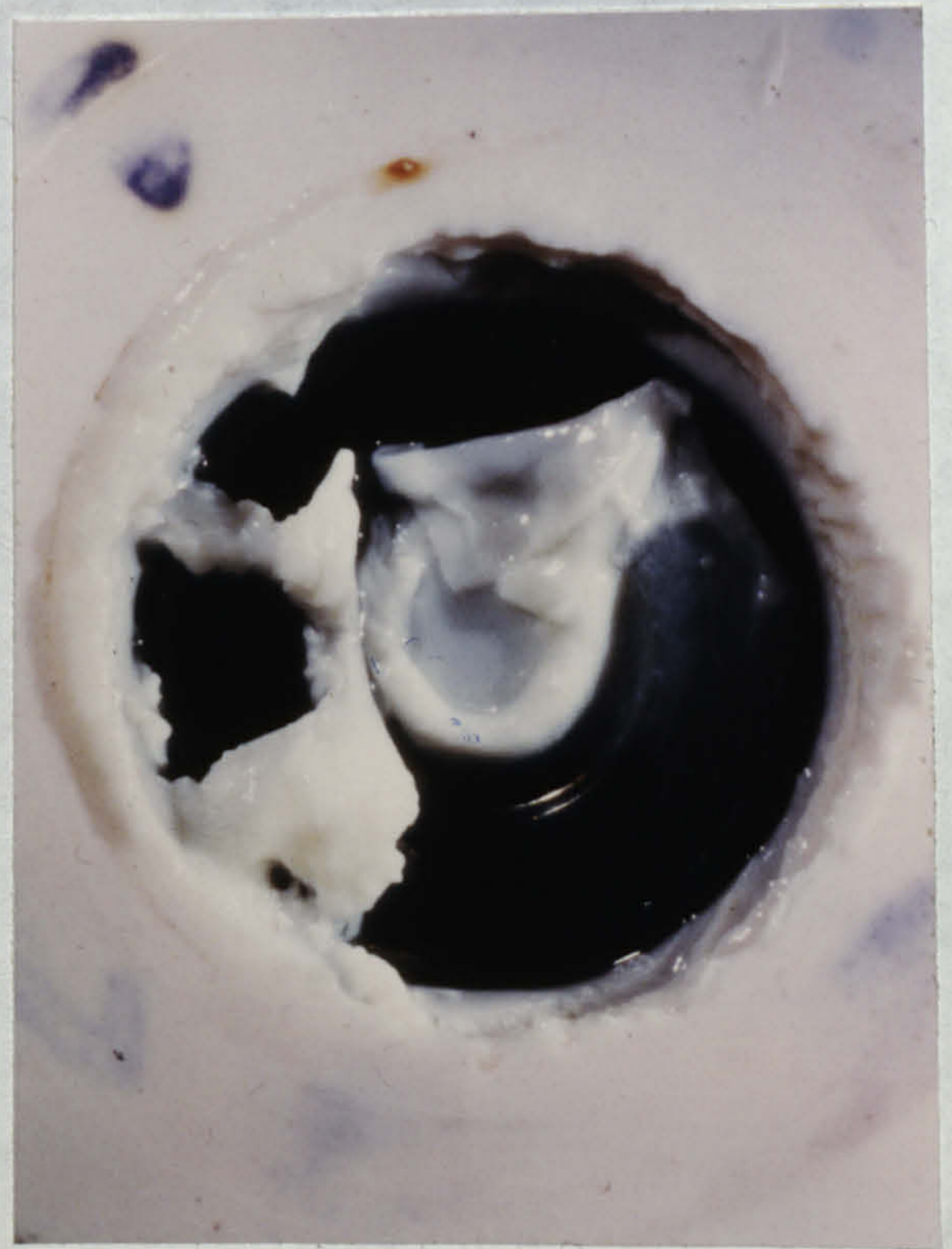
Fig 82. Milk. Bjork-Shiley Aortic Downstream. 40°C. 3L/min milk
