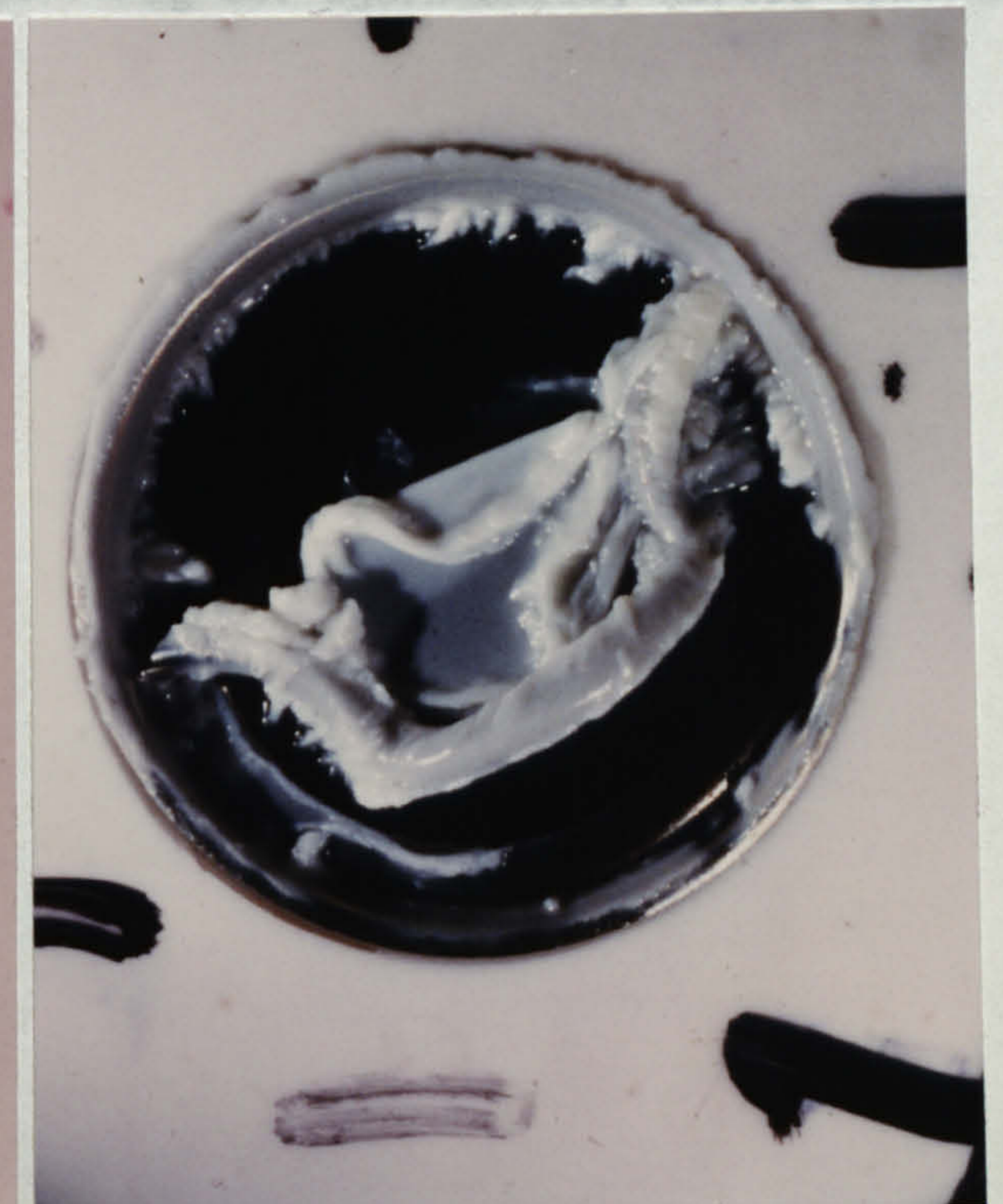
Fig 64. Bjork-Shiley Aortic Upstream 40°C. 3L/min milk.
