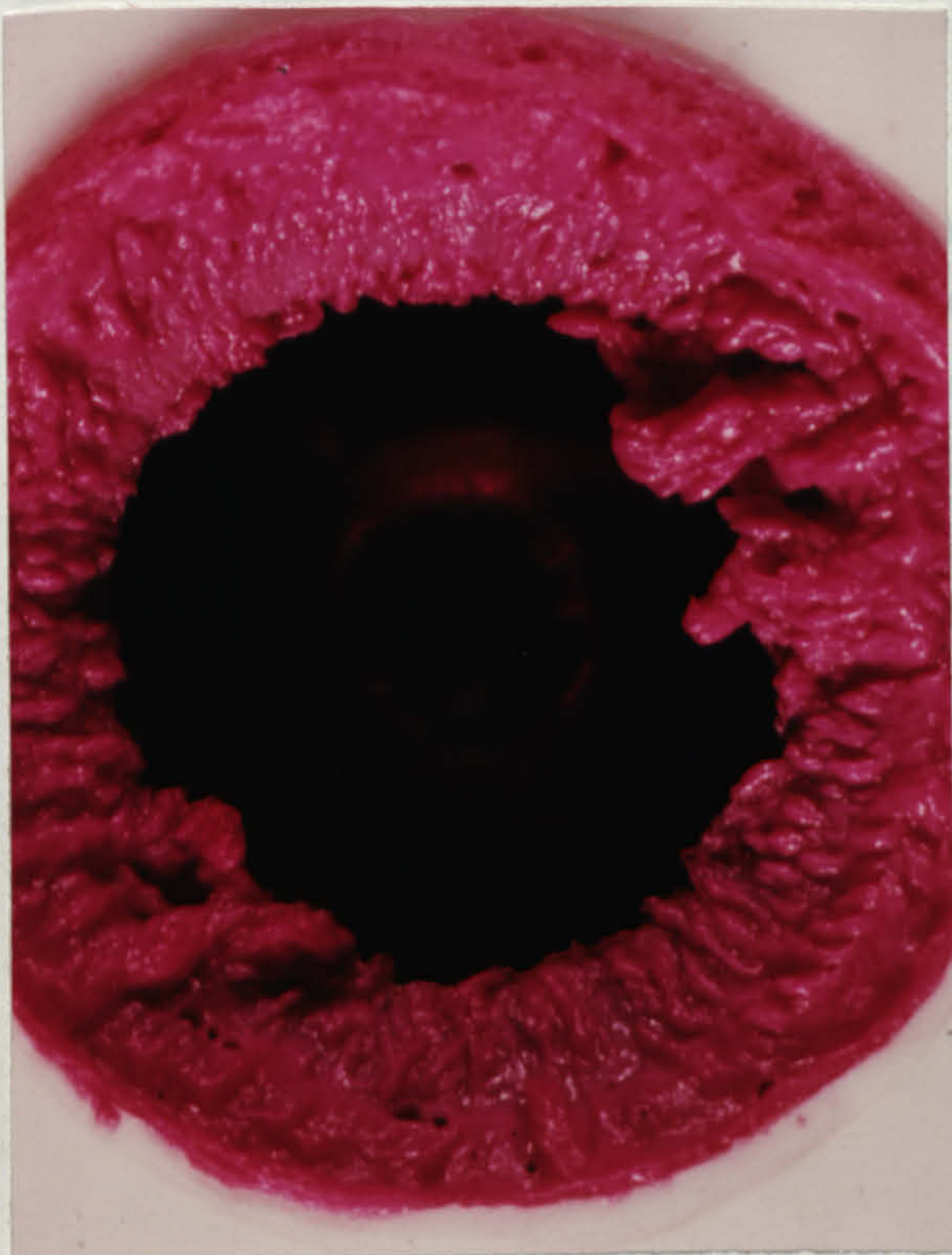
Fig 145. Starr-Edwards Mitral Upstream 40°C. 2L/min milk
