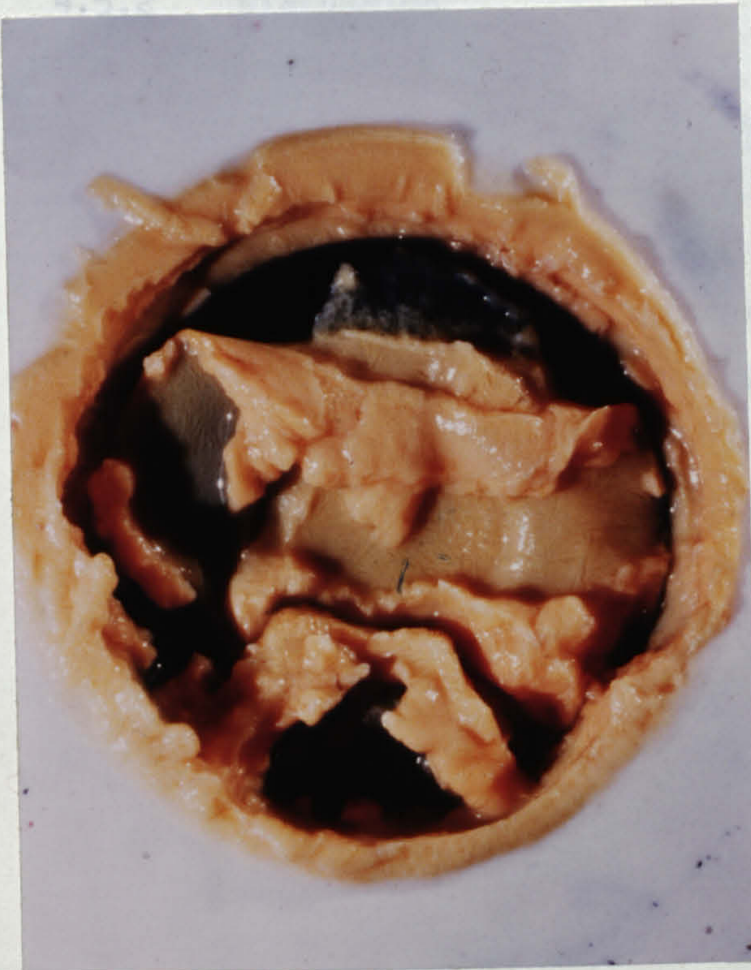
Fig 71. Bjork-Shiley Aortic Downstream. 39°C. 3L/min milk.
