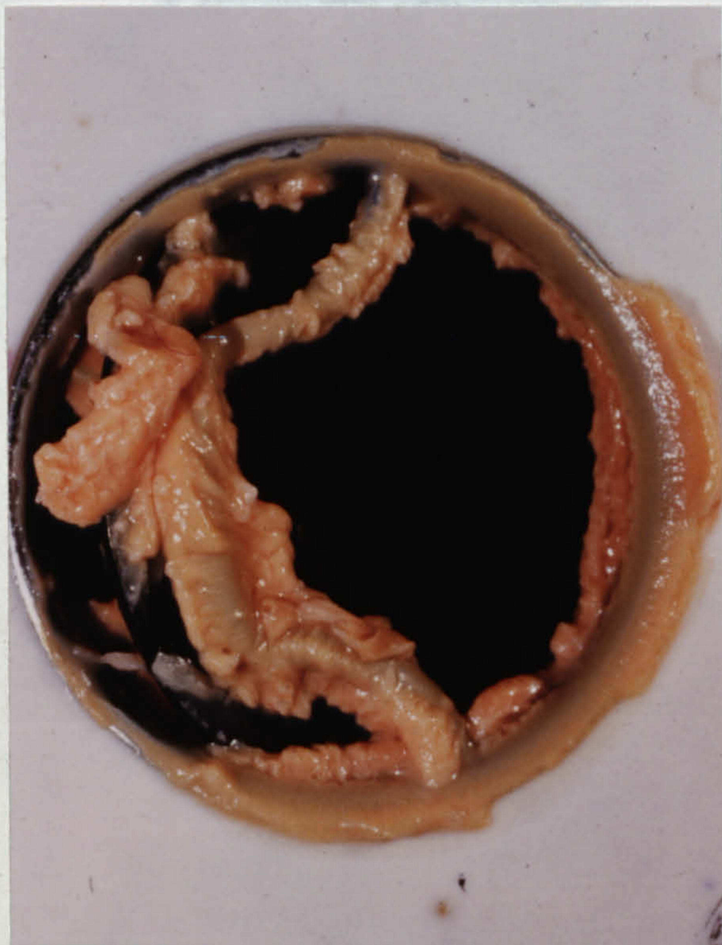
Fig 65. Bjork-Shiley Aortic Upstream 39°C. 3L/min milk.
