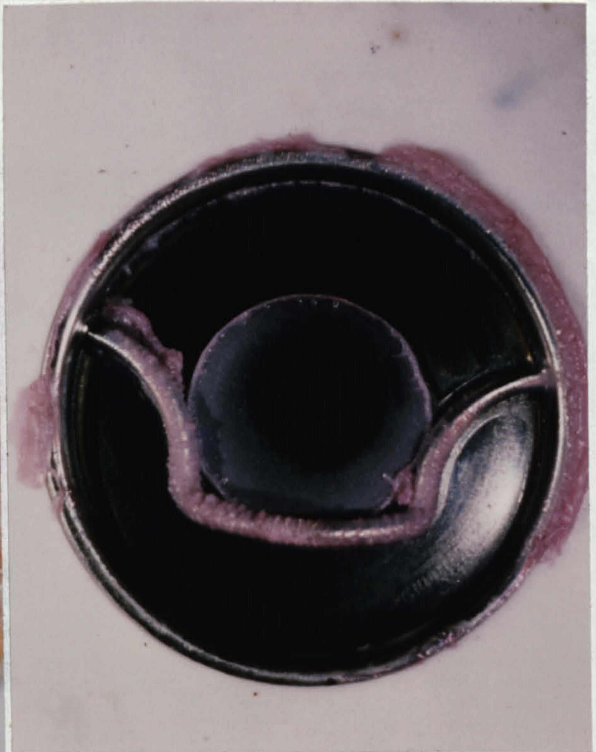
Fig 114. Bjork-Shiley Aortic Upstream 38°C. 3L/min milk.
