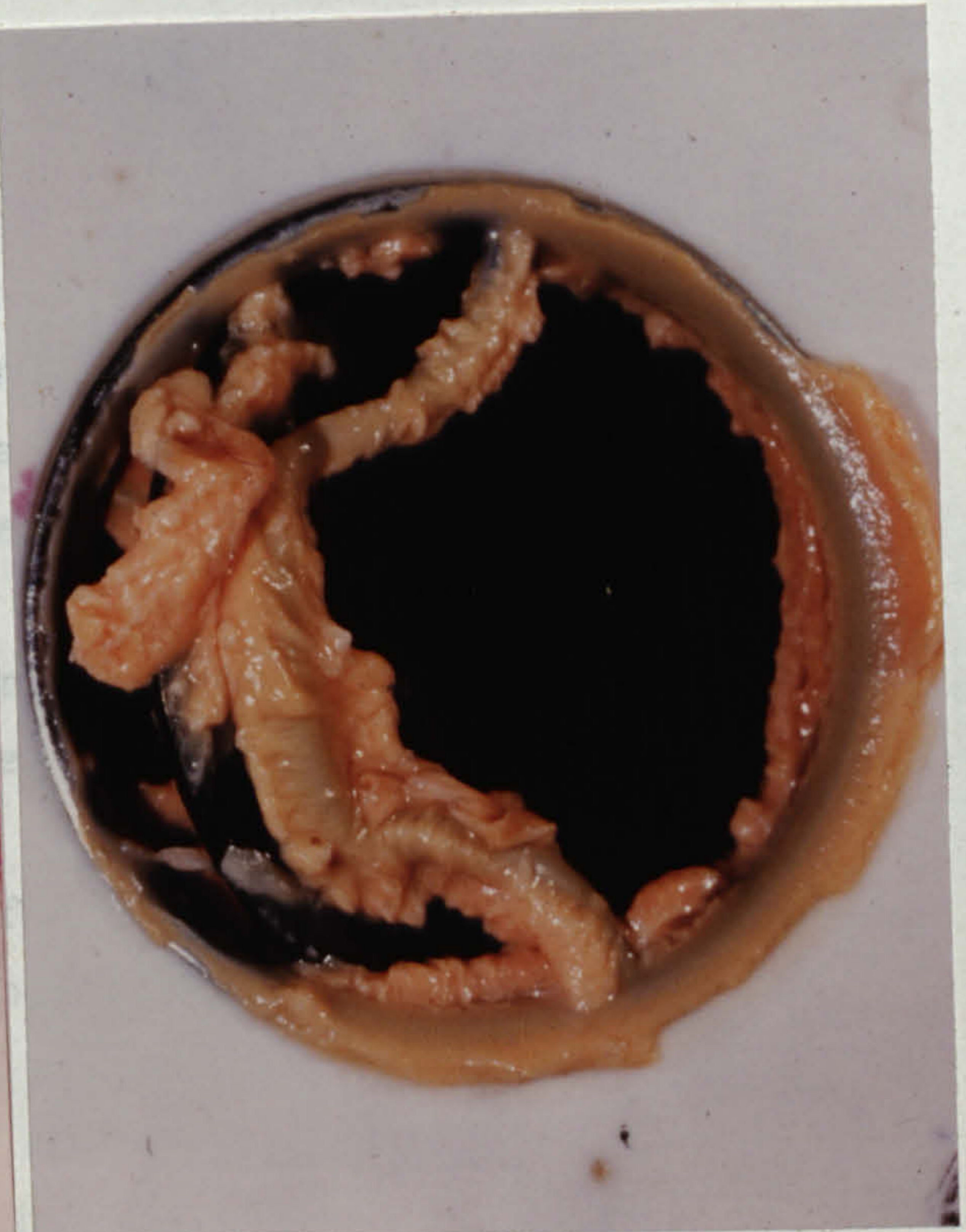
Fig 116. Bjork-Shiley Aortic Upstream 39°C. 3L/min milk.
