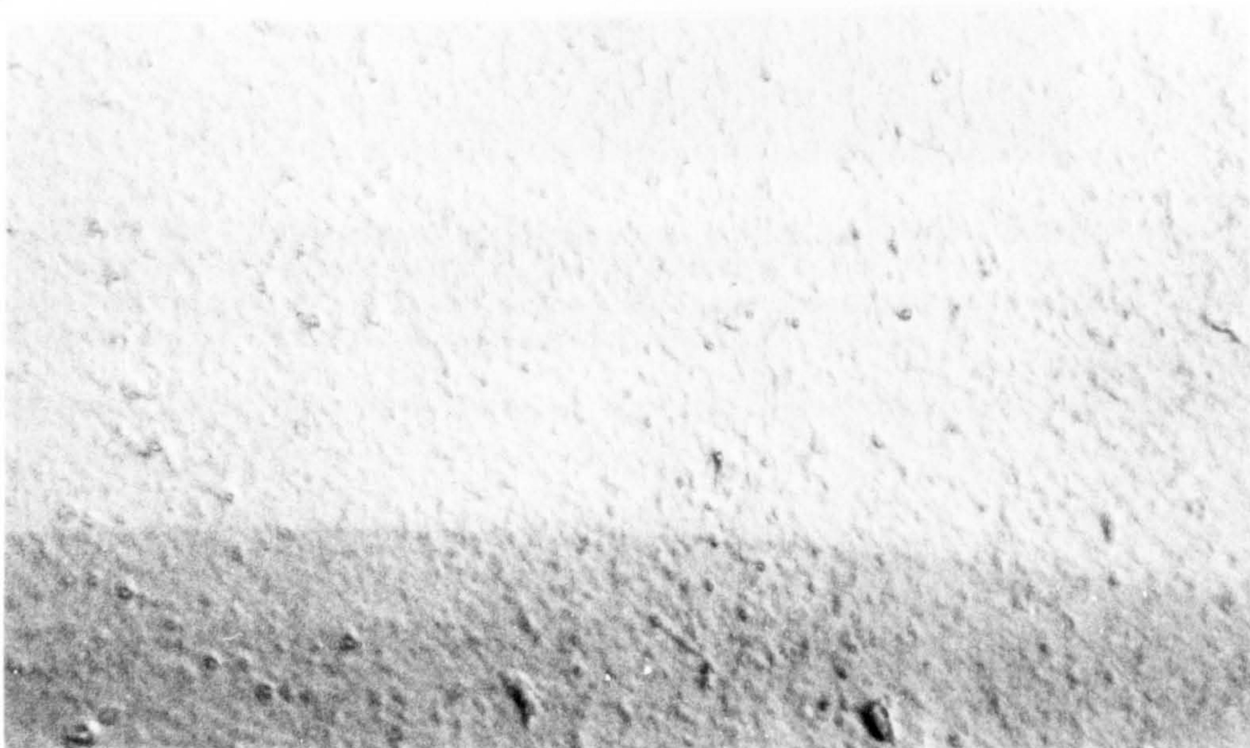
Fig 16. Milk. Slide surface outside stagnation point after run. Standard chamber has hole diameter of 2,5mm and a distance of 0.31mm between the chamber column and the slide giving a \beta value of 17(\text{mm sec})^{-1} . The milk flow rate is 2ml/min throughout and rennet and cone \text{CaCl}_2 solution are both added to 1% by volume. The run duration was 5 minutes and the temperature 38^\circ\text{C} . Magnification 840x.
