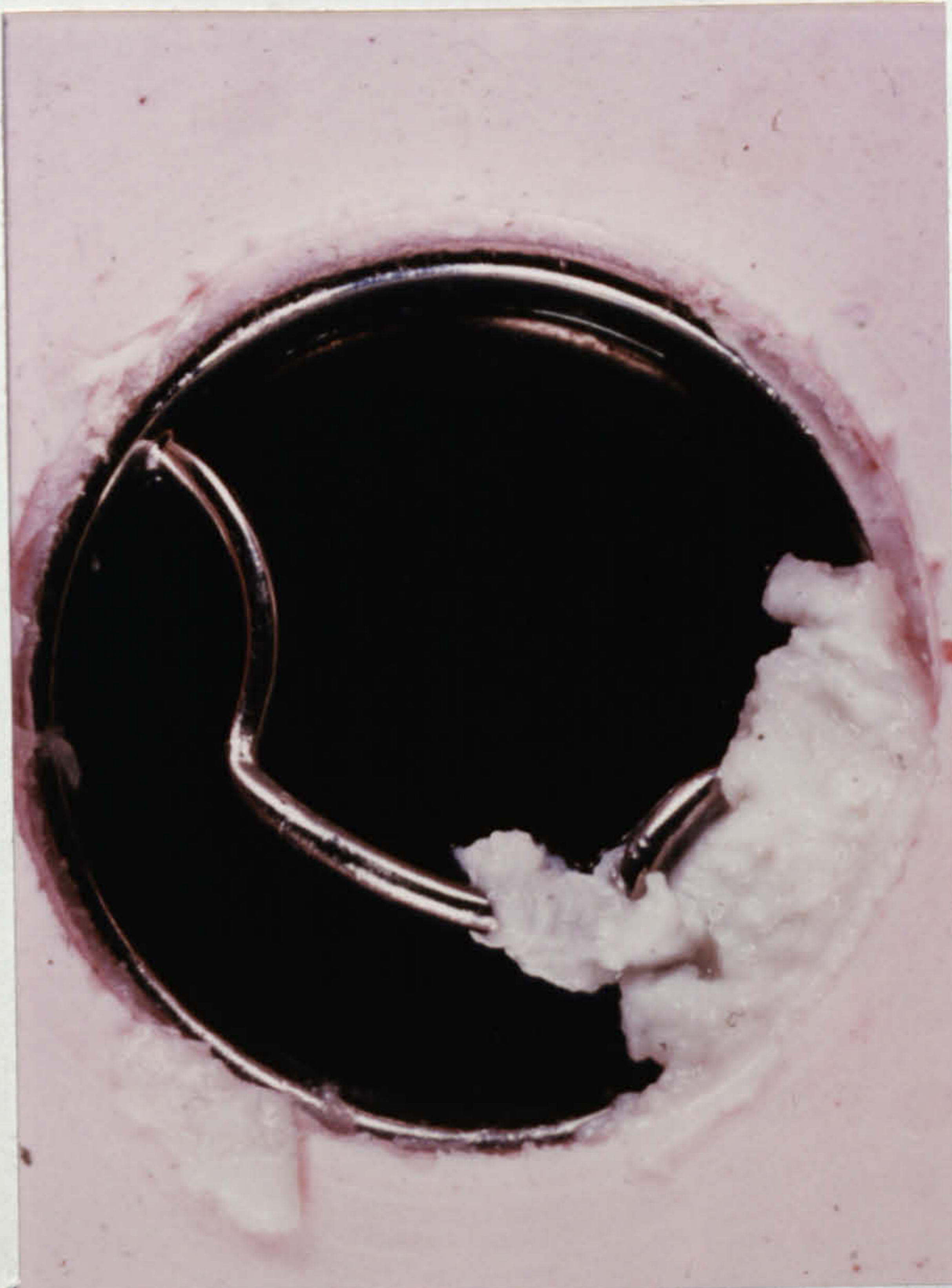
Fig 61. Bjork-Shiley Aortic Upstream 40°C. 0.6% CaCl 2 & rennet. 2L/min milk. Valve albumen coated.
