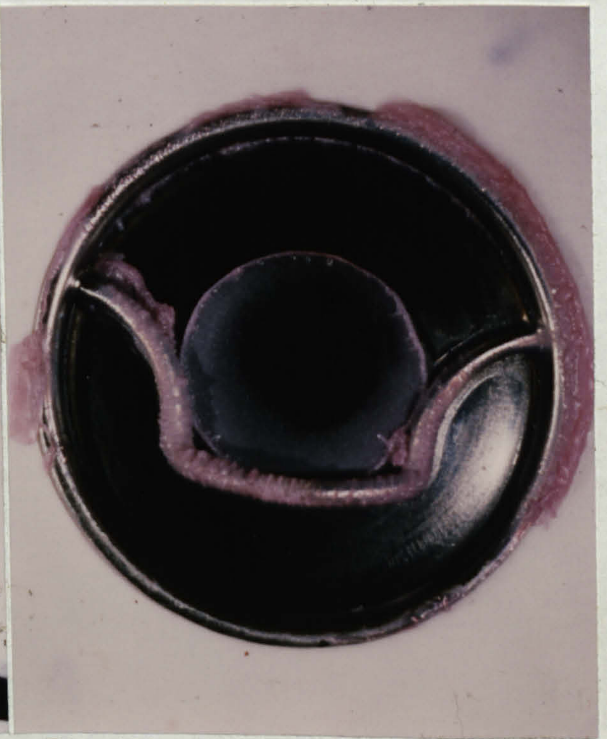
Fig 152. Bjork-Shiley Aortic Upstream 37°C. 3L/min milk
