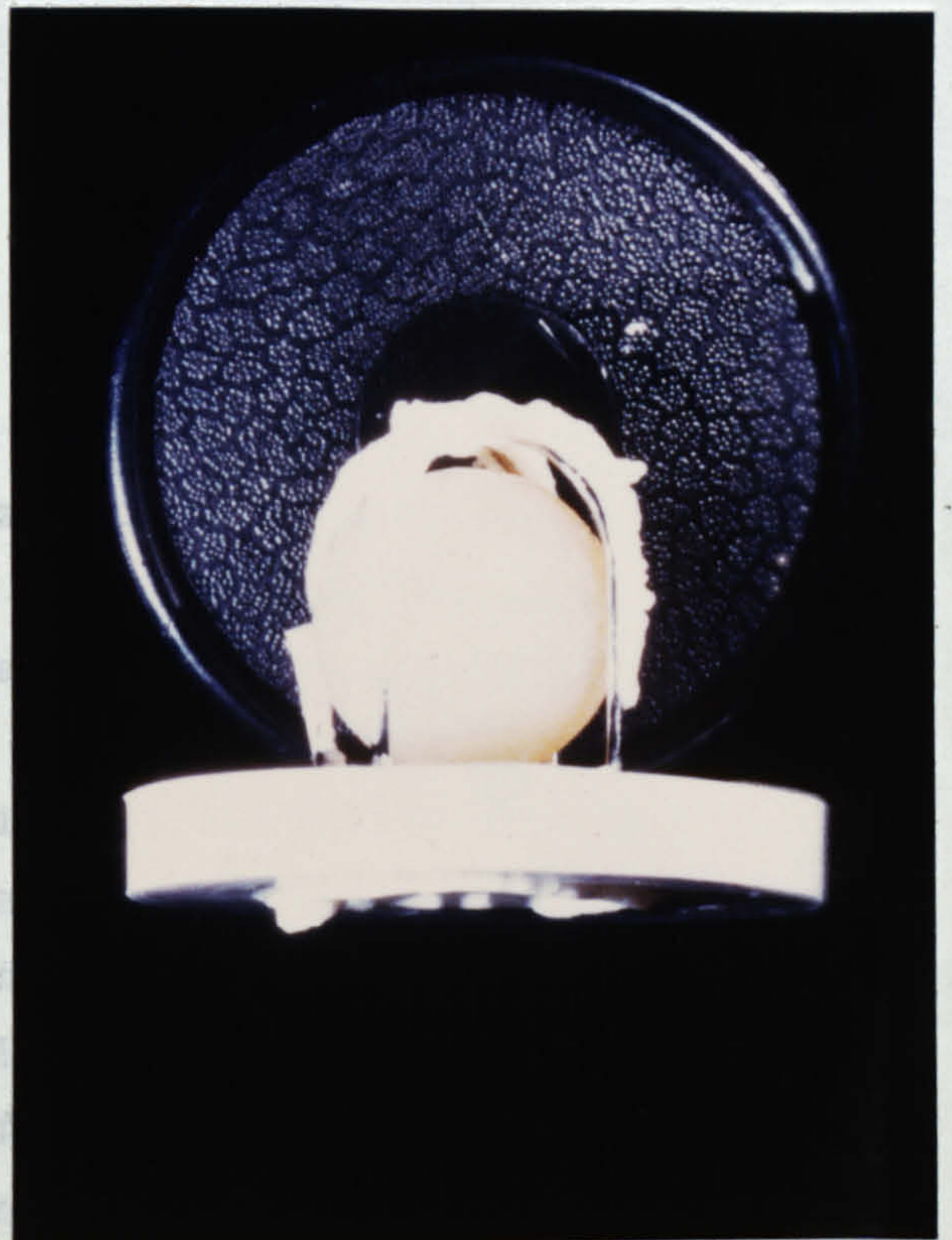
Fig 91. Milk. Starr-Edwards Aortic Downstream. 38°C. 2L/min milk.
