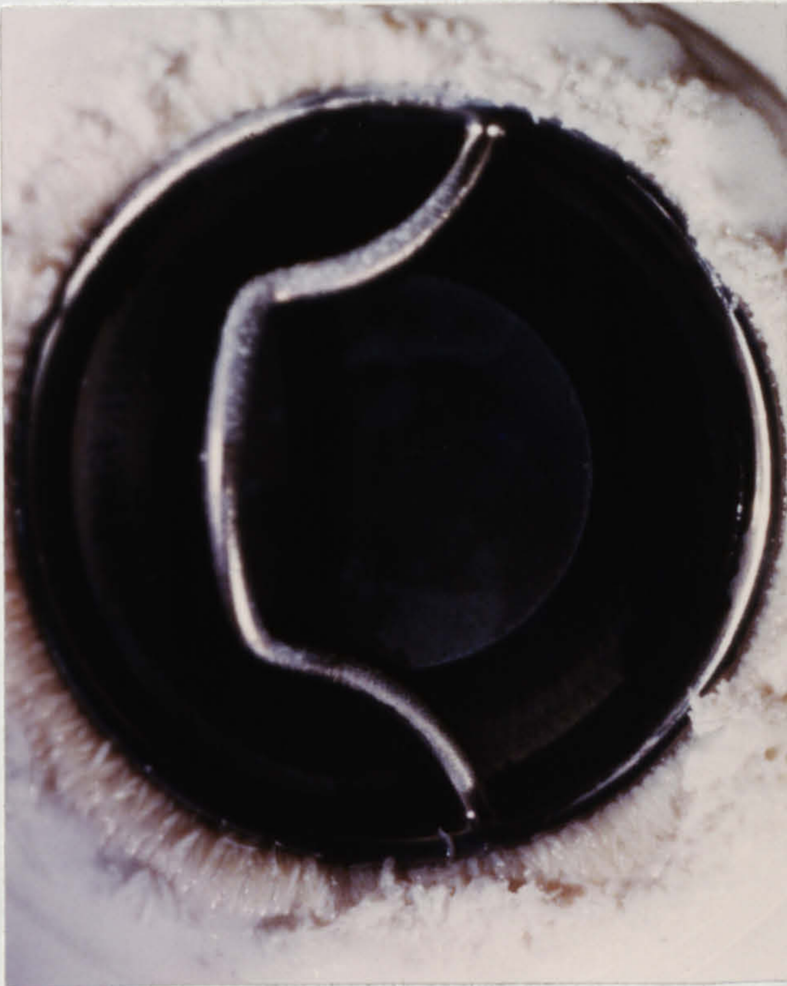
Fig 139. Bjork-Shiley Mitral Upstream 40°C. 3L/min milk
