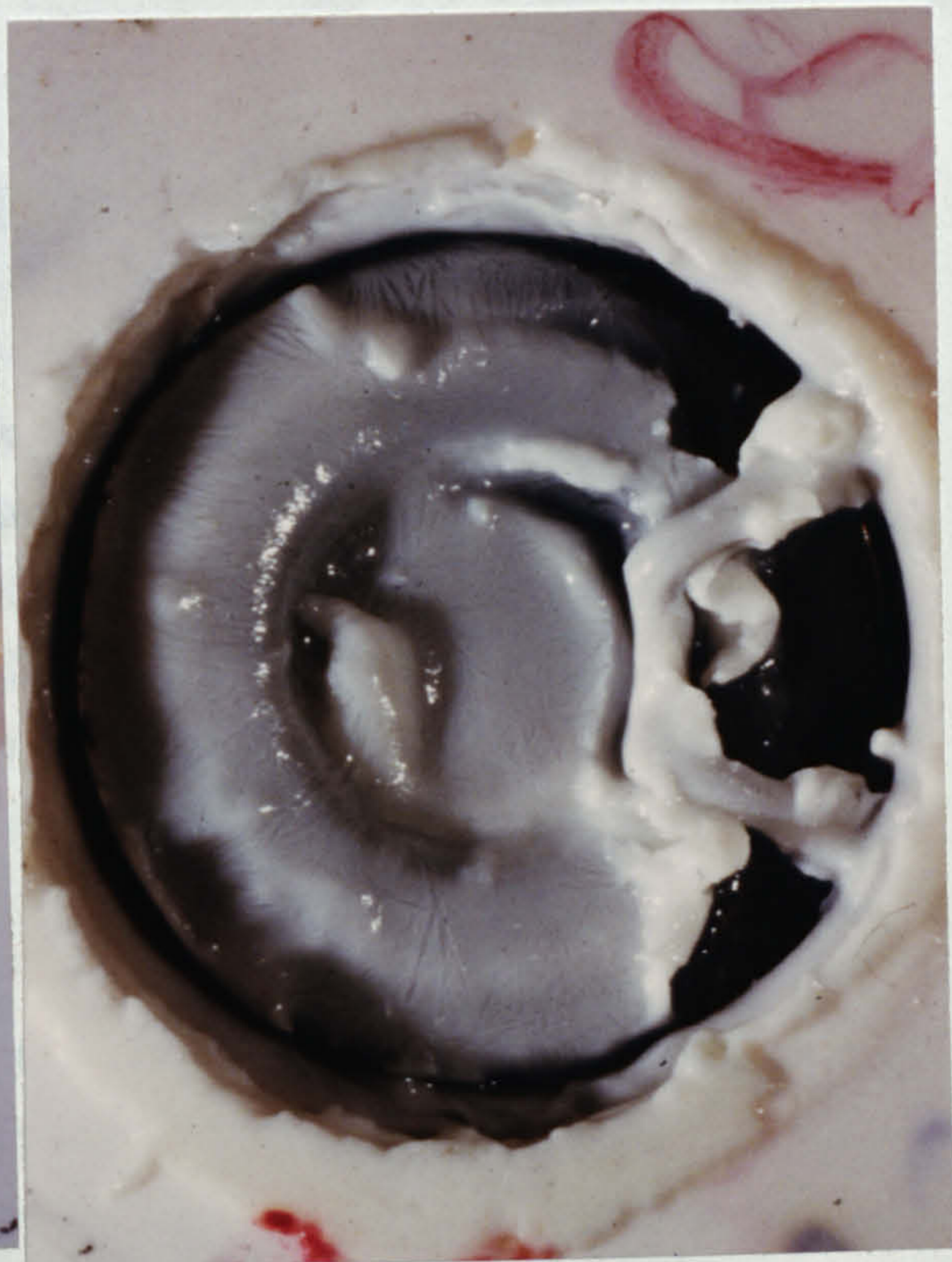
Fig 72. Bjork-Shiley Aortic Downstream. 38°C. 3L/min milk.
