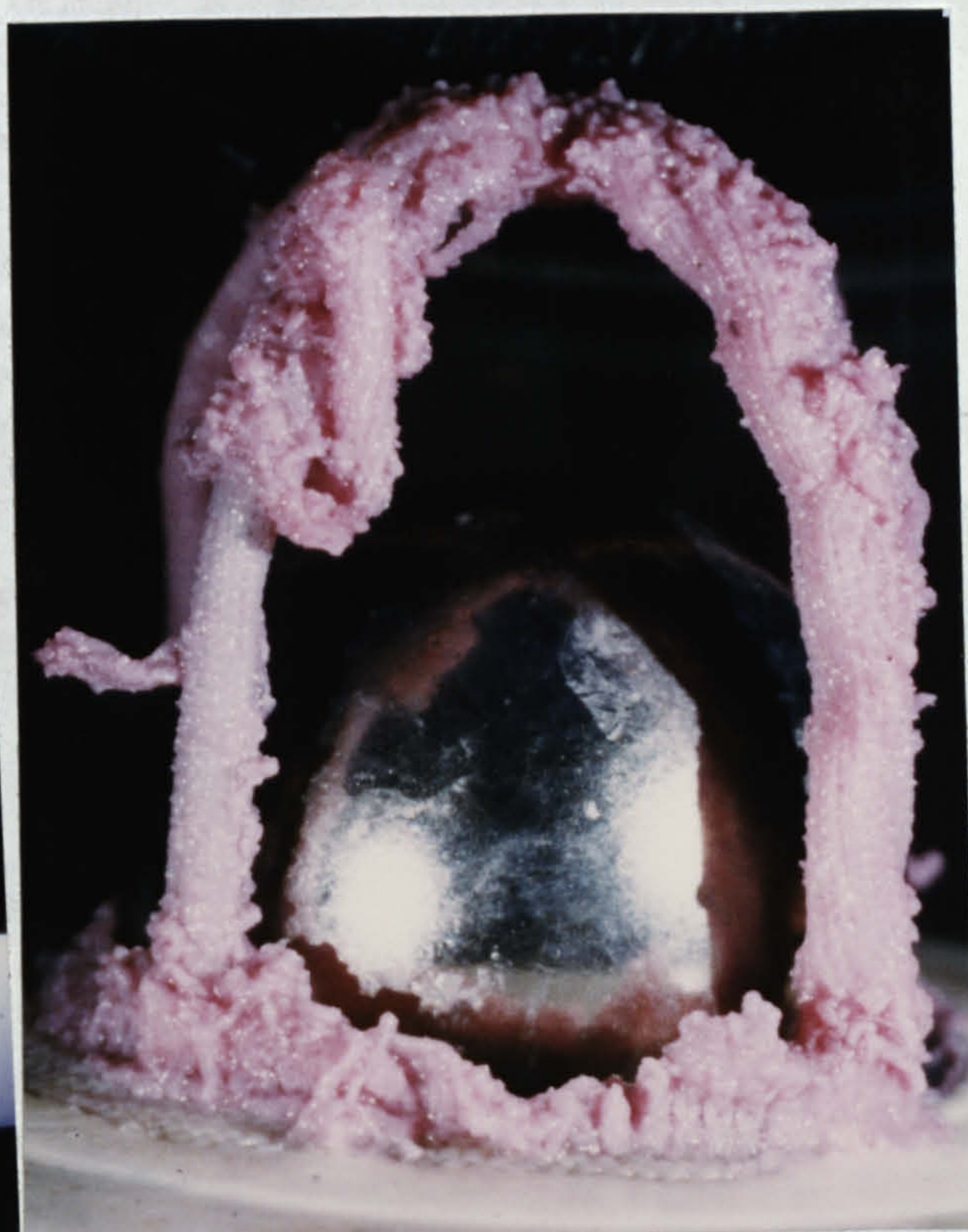
Fig 60. Starr-Edwards Mitral Downstream. 38°C. 3L/min milk.
