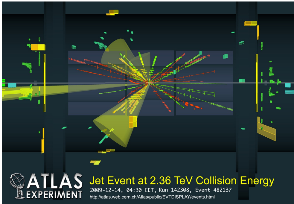
Figure 4.1 An event display from a collision recorded by the ATLAS detector [121]. The yellow cones indicate energy deposits that have been clustered together and identified as jets.
