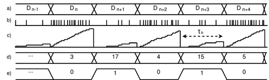
Fig. 3. Timing diagram showing (a) input data, (b) pixel SPAD pulses, (c) counter iteration during \tau_b , (d) latched 6b data, and (e) data output post threshold.
