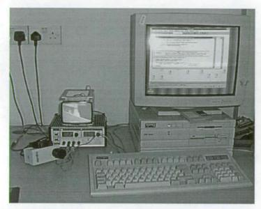
Figure 4.13 The PINK FPGA test set-up. The imputer system (containing the FPGA), the power supply and monitor can be seen to the left of the PC.
