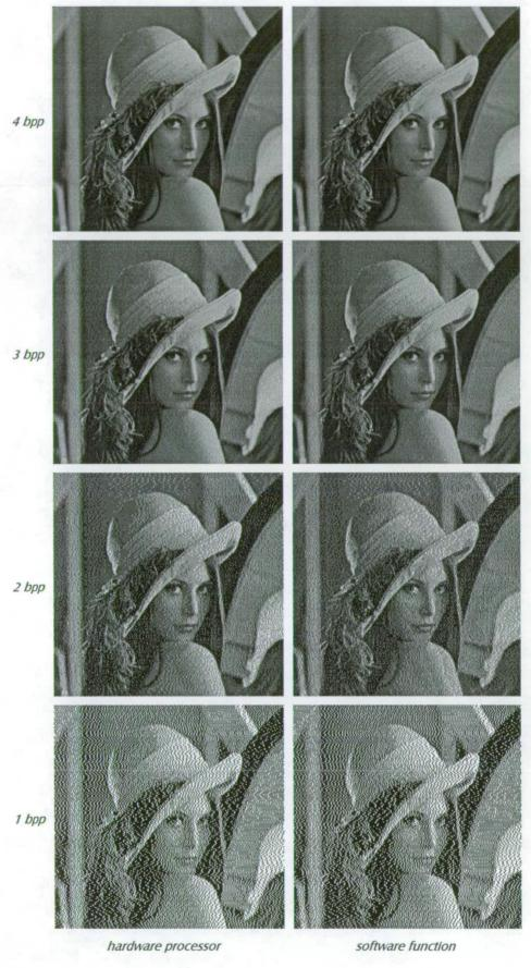
Figure 4.17 Comparison of the output of the hardware 'simple' processor with that of its software counterpart.
