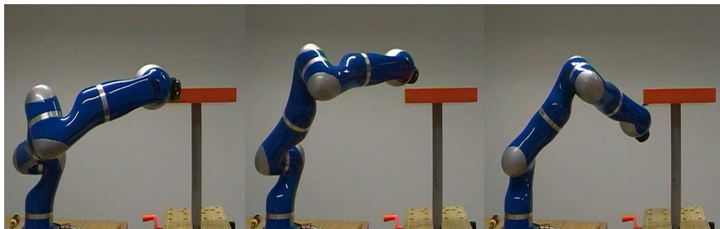
Figure 5.11: Anthropomorphic DLR/KUKA light-weight arm (LWR-III) in reaching experiment.
