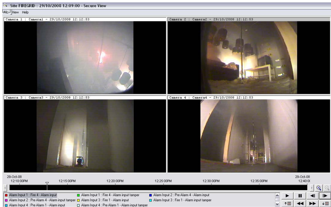
Fig. 3. Four camera view of full-scale demonstration test – 4 minutes after heat detector alarm
