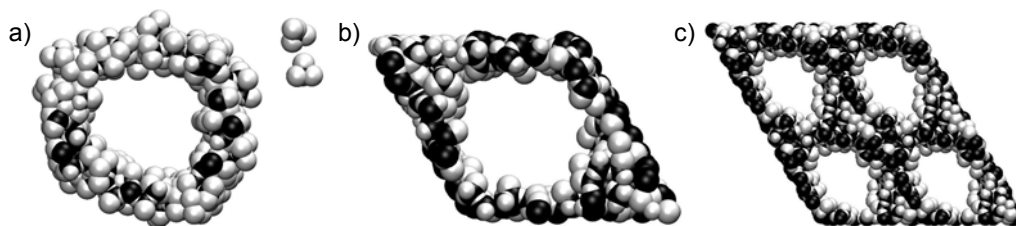
Figure 6-9 Snapshots from the kMC simulation with a potential based on the micelle with the HH_6 T_{10} surfactant. a) At the beginning of the simulation; b) during aggregation and c) the calcined sample (four unit cells).
