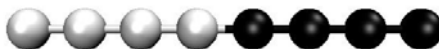
Figure 6-3 Representation of the linear surfactant used with four head (black) and four tail (grey) segments.
