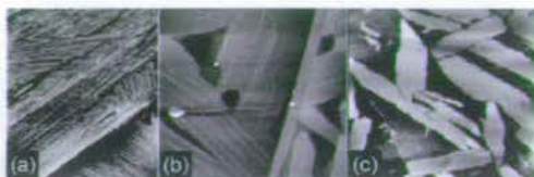
FIG. 2. Meso-scale FM-AFM images of an EFR thin film on HOPG (a) in UHV before annealing ( 464 \text{ nm} \times 558 \text{ nm} , cantilever: Nanosensors NCH, \Delta f = -15 \text{ Hz} , a = 8 \text{ nm} ), (b) in UHV after annealing ( 500 \text{ nm} \times 500 \text{ nm} , cantilever: NCH, \Delta f = -20 \text{ Hz} , a = 8 \text{ nm} ), (c) in ambient conditions no annealing ( 500 \text{ nm} \times 500 \text{ nm} , cantilever: Nanosensors EFM, \Delta f = -25 \text{ Hz} , a = 9.6 \text{ nm} , Q = 154 ).
