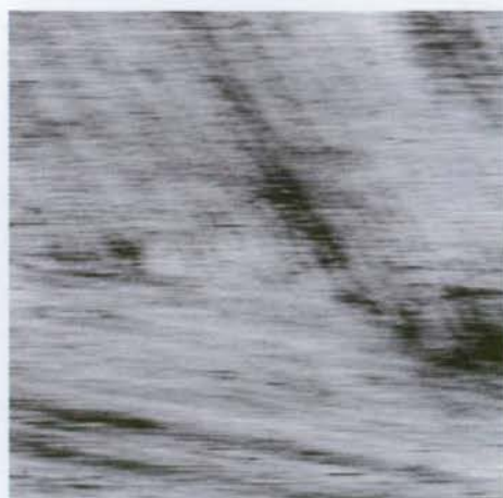
FIG. 5. Molecular-scale ambient FM-AFM topography image of EFR thin film on HOPG ( 70\text{ nm} \times 70\text{ nm} , cantilever: Nanosensors NCHR+magnet, a = 10.8\text{ nm} , \Delta f = -35\text{ Hz} ).
