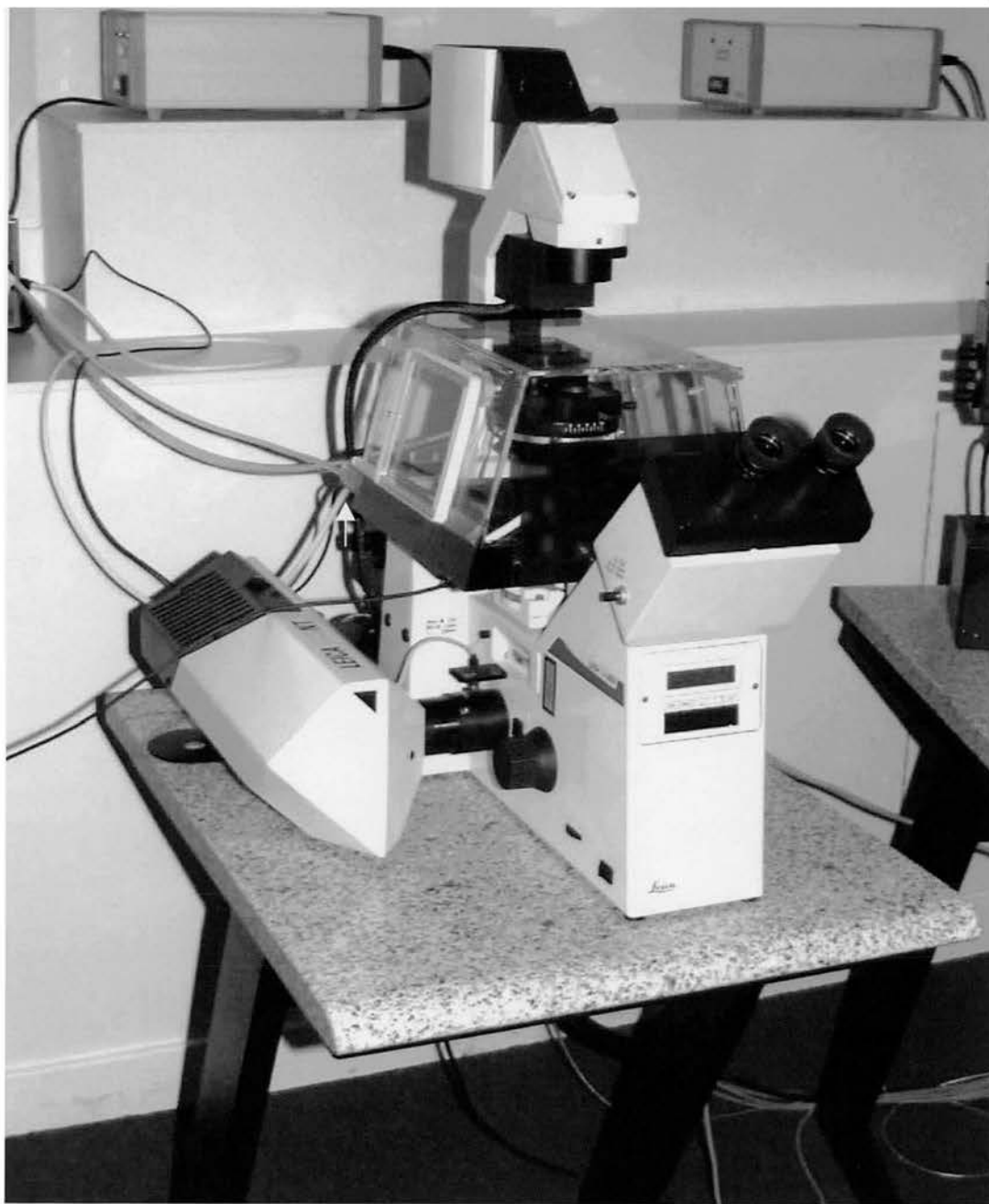
Fig 3.3 The Leica Incubation Chamber for time-lapse confocal microscopy. The plastic tube on the left hand side (arrow) is attached to an infra-red gas monitor (not in view), to sample the CO 2 level. CO 2 is pumped into the chamber from the plastic tube on the right hand side of the chamber when the level drops below 5%.
