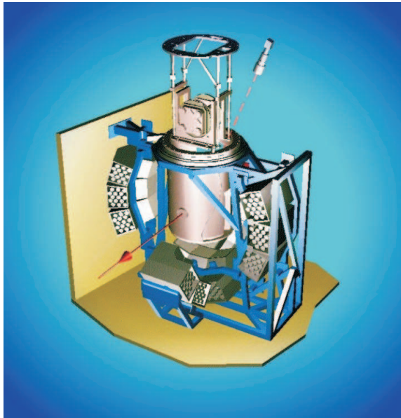
Figure 3.18: Showing the PEARL/HiPr instrument and how the Paris-Edinburgh press is mounted into it. (a) shows a representation of the instrument itself, the red arrow indicates the directions of neutrons through the instrument. There are two banks of detectors, the first is in a traverse geometry and the second in a longitudinal geometry. The press is centred into the instrument in a two staged process. The first of this is the vacuum jacket tank, and then a cradle which fits into the tank. (b) shows a Paris-Edinburgh press in place on a cradle. The press is fitted with centring rings which allow the sample to be rotated, usually to avoid obscuring by the cell ti rods.
