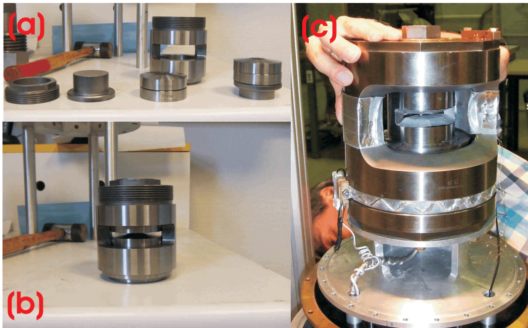
Figure 6.2: Images of the sample clamp for the Paris-Edinburgh press. The parts that make up the apparatus are illustrated in (a), there are two anvils, two backing disks, two plugs and a holding ring that fit inside the body of the clamp. The apparatus is assembled in (b). Load is applied to the upper plug and pressure is generated at the sample. Once the load is applied the holding ring (which has a thread to attach it to the clamp body) is screwed to hold the pressure in the clamp. The plugs on both the top and bottom of the clamp means that once the clamp is placed into the Paris-Edinburgh press (c) further load can be applied to the sample.
