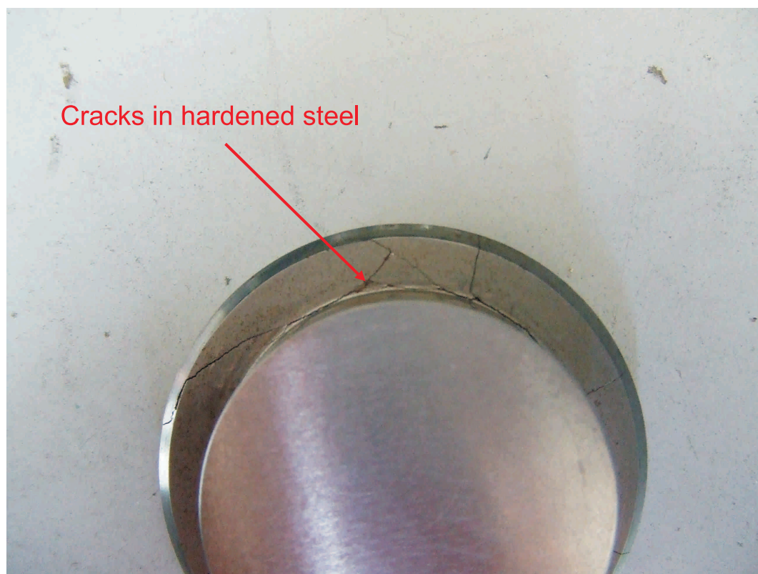
Figure 6.3: The top plug of the clamp which was damaged during the ILL experiment.
