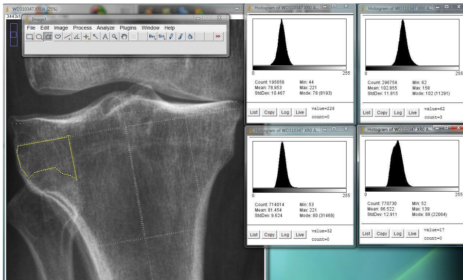
Figure 2.8 Preoperative radiograph analysis. The 4 ROIs have been delineated with exclusion of the fibular head and cortical condensations using Image J. The measurement D4 has been used to ensure the ROIs are at the same depth as in the postoperative radiograph in Figure 2.9. Adjacent histograms indicate the greyscale measures for each ROI.
