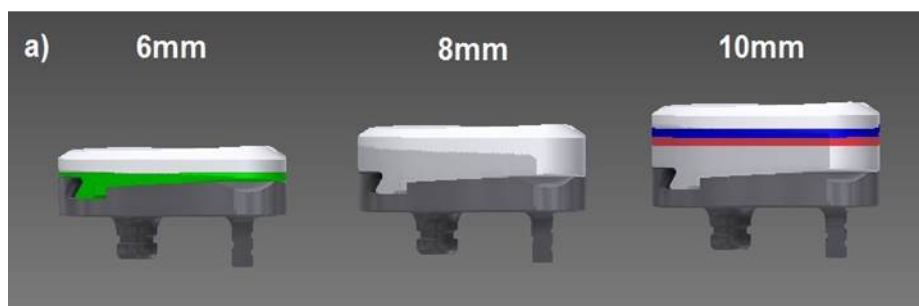
Figure 2.35 MB tibias of different thickness created from the original 8mm implant. The red and blue sections represent 1mm thickness additions. 2mm has been removed from the superior surface of the green part to create the 6mm implant.
