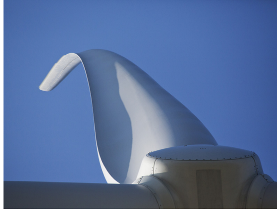
Figure 4.1: Aeroelastic deflection of a wind turbine blade. After Siemens [205].
