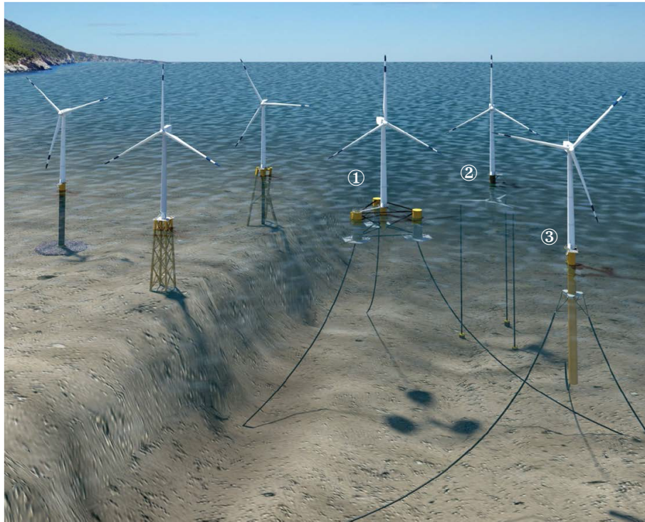
Figure 1.3: Bottom-fixed and floating offshore wind turbines, after Smith et al. [11].
