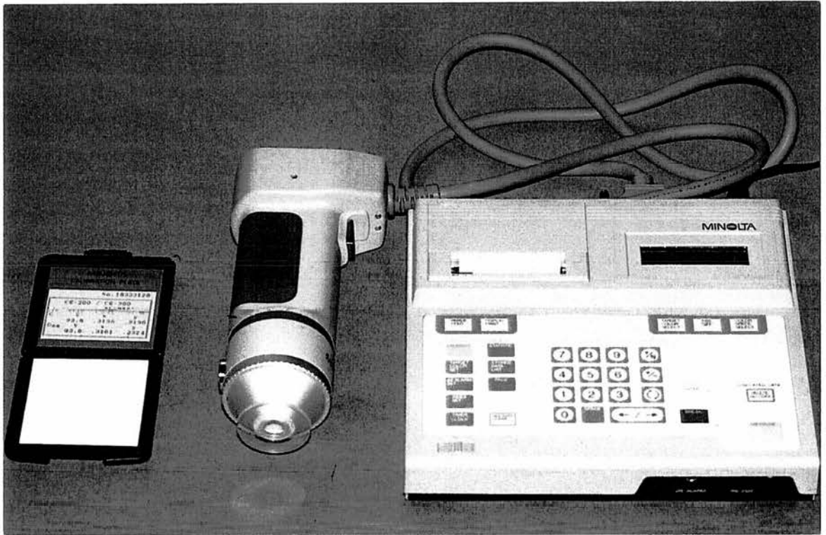
PLATE 2.5 Minolta CR-300 Chroma meter with adjacent white calibration tile
