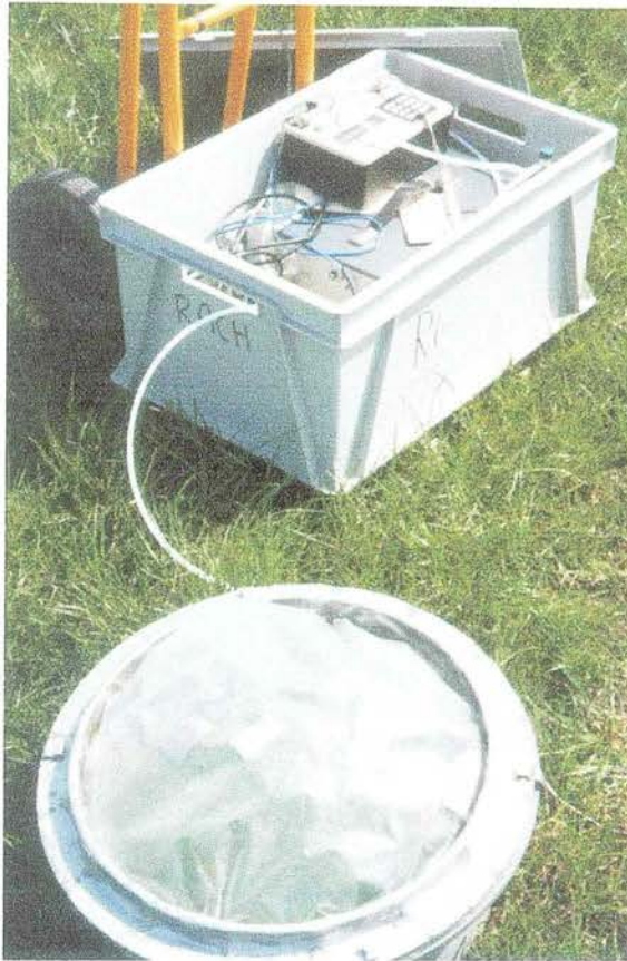
Plate 4.1 Gas sampling system using the Scintrex analyser
