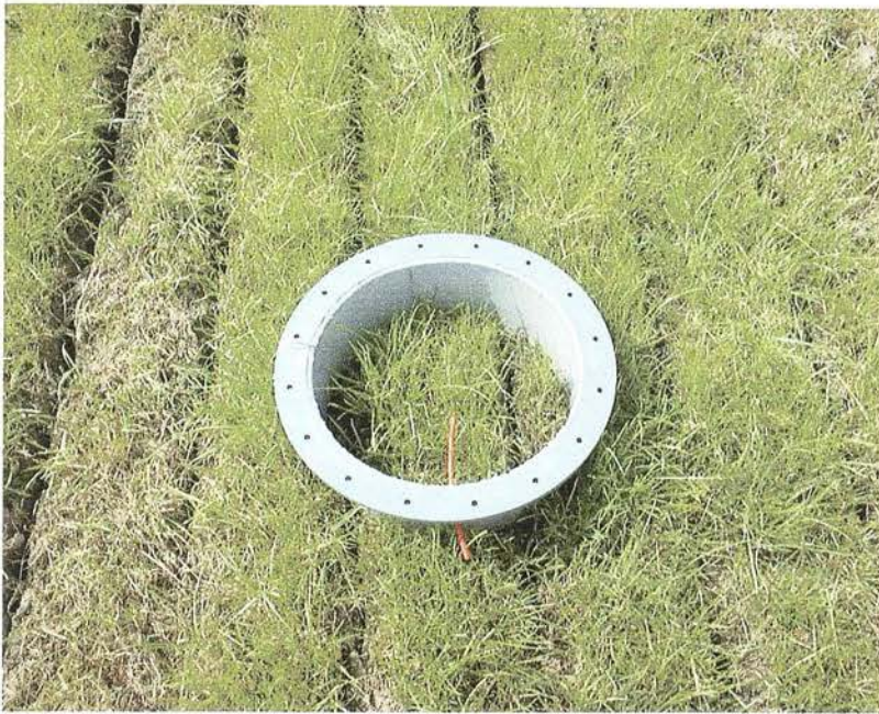
Plate 4.3 Chamber positioned over injection slots on the cattle slurry treatment
