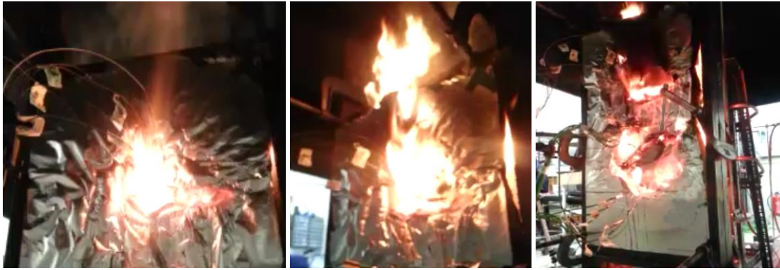
Figure 7.39. Evolution of the back face of the insulation board tested at 65 \text{ kW}\cdot\text{m}^{-2}
