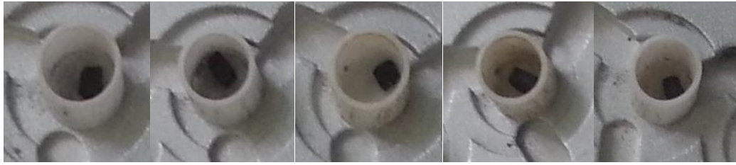
Figure 4.5. Examples of remaining char after TGA tests in a nitrogen atmosphere
