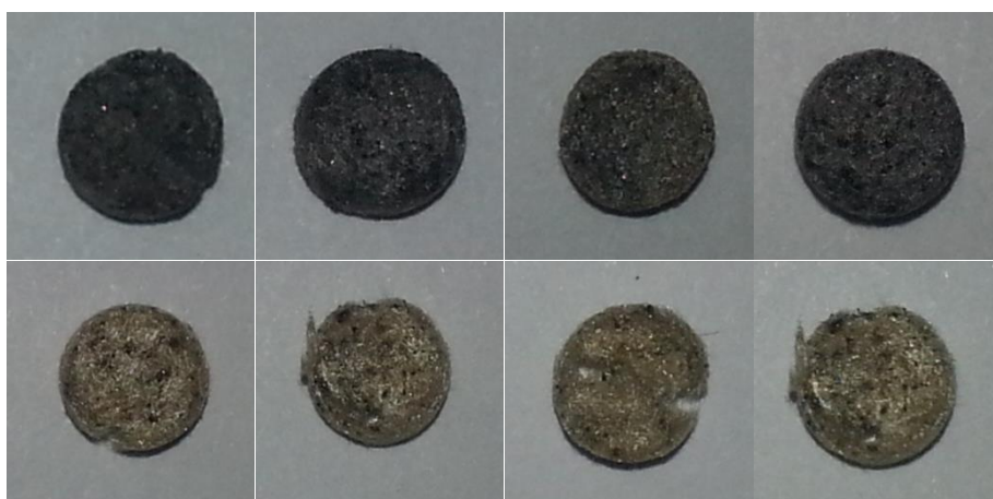
Figure 4.4. Examples of stone wool residue after TGA tests in a nitrogen atmosphere (top) and air (bottom)
