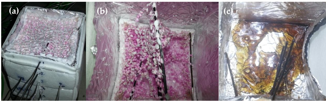
Figure 6.18. EPS sample residue at (a) 2 kW·m -2 , (b), 4 kW·m -2 and (c) 10 kW·m -2
