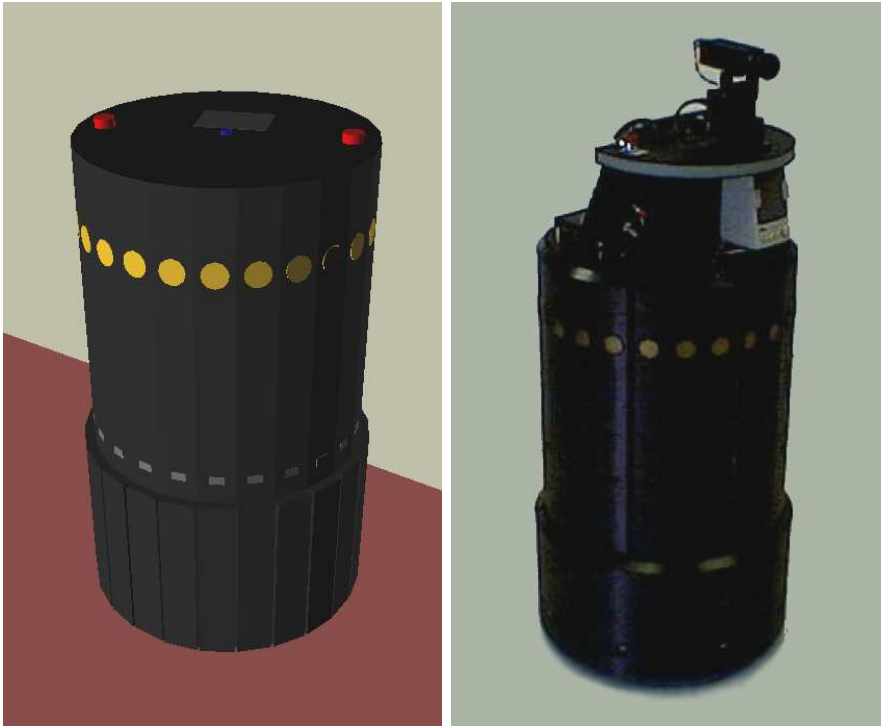
Figure 8.7: Simulated model B21 robot and its real counterpart “Gillespie”
