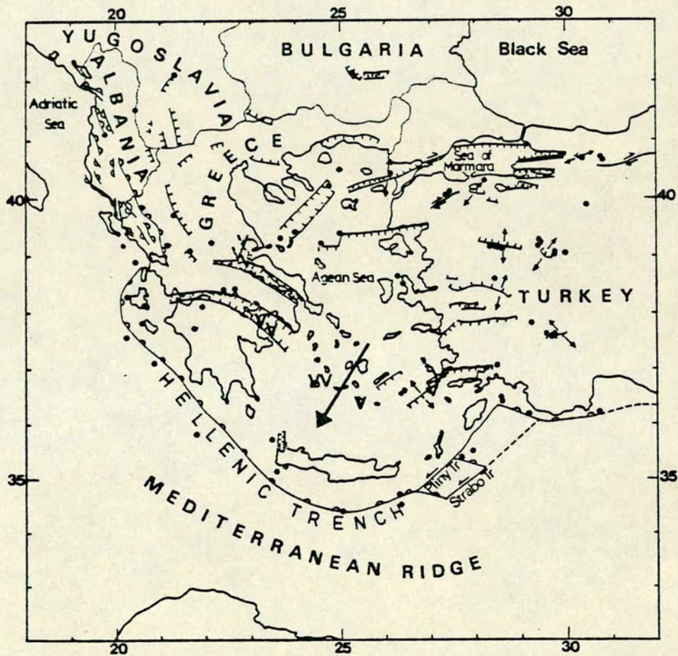
Fig 6-4 Summary of the present deformation of the Aegean area after McKenzie (1978). (Long curved lines show normal faults. Lines with open semicircles show thrust faults. Solid dots mark epicenters of shocks for which mechanisms are used. Arrows show the direction of motion obtained from fault plane solutions. The long heavy arrow shows the direction of relative motion between the Aegean and Africa. Heavy Vs mark sites of recent volcanism.)
