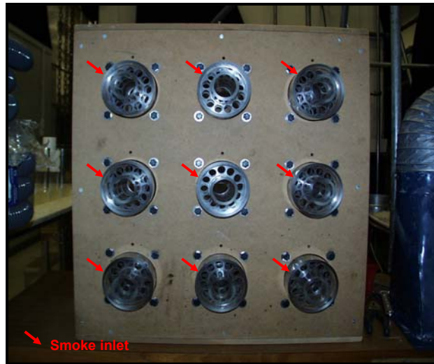
Figure 5.2 Points of smoke injection into the airflow
