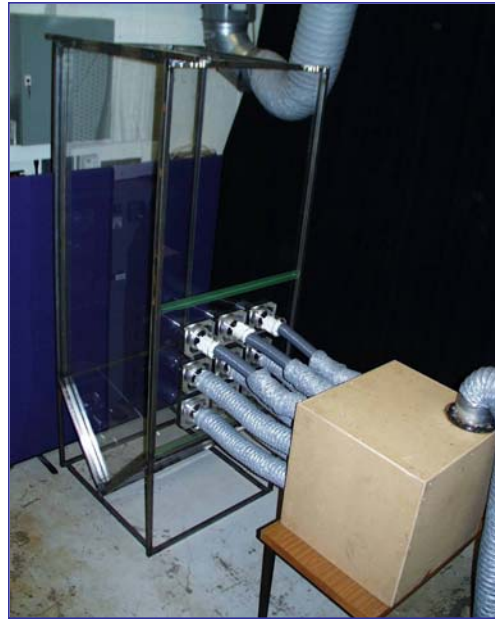
Figure 4.9 Furnace and windbox assembly
