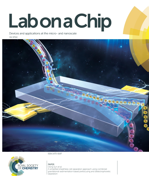
Figure 1.3: Cover page from the journal “Lab on a Chip”, a leading journal of microfluidic technologies. The image illustrates bi-modal separation of two types of cells using a modified microfluidic dielectrophoresis (DEP) device. The article describing the details of the microfluidic device is referenced in the cover image. Reproduced with permission from ‘Front cover’ (2018) (©RSC).
