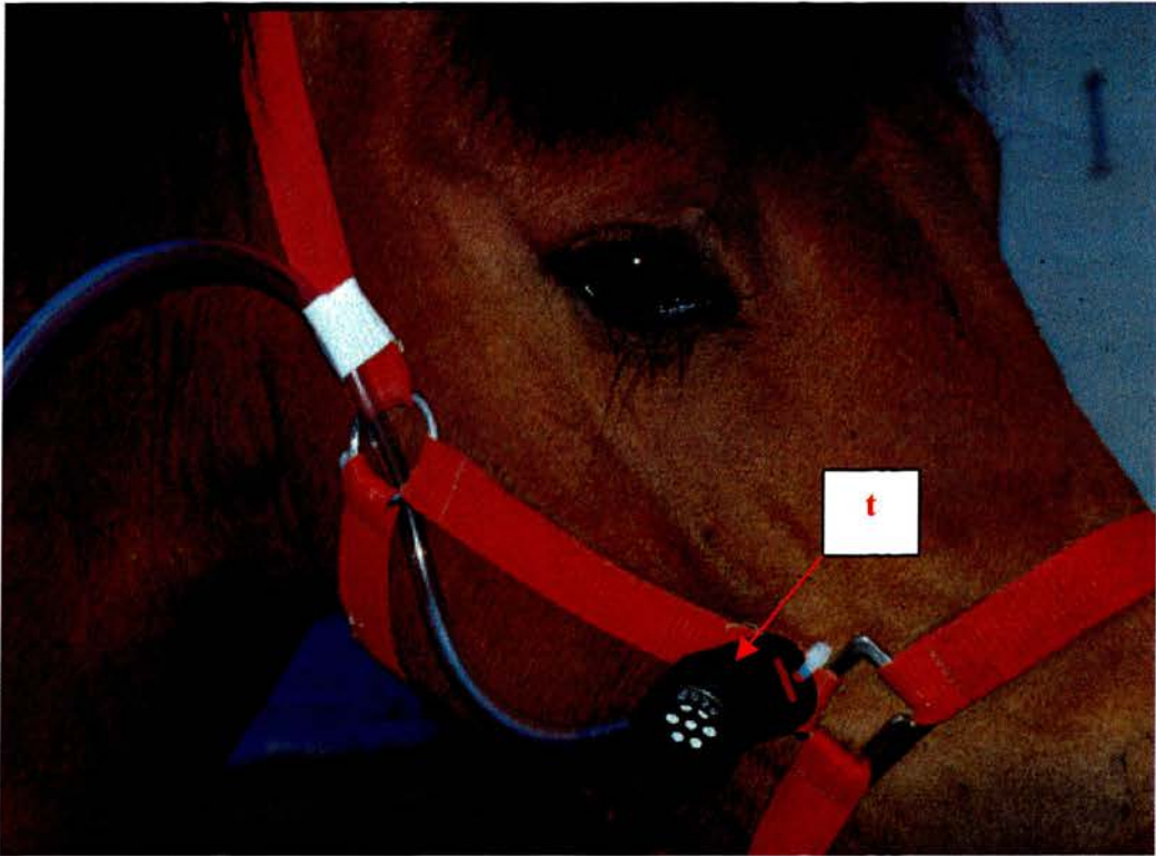
Fig. 2.4: A sampling head designed for collection of total airborne dust (t) was attached to to the right side of the head-collar in order to collect from the horses breathing zone
