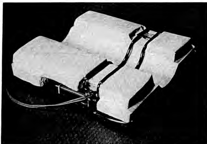
Fig. 2. Prototype breast coil showing the surface coil shaped to fit round the breast when the patient lies prone on the coil support. The curvature of the coil is sufficient for a wide range of breast sizes to be imaged.
