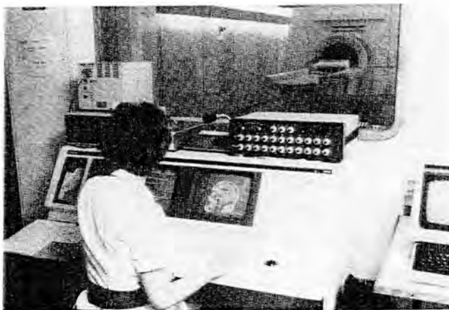
Figure 4 The 1.5 T Gyroscan Magnetic Resonance Imaging and Spectroscopy system manufactured by Philips Medical Systems. In the foreground the operator can be seen in front of the control console on top of which is the box used to adjust the magnet shim. Through the window can be seen the patient couch and magnet
